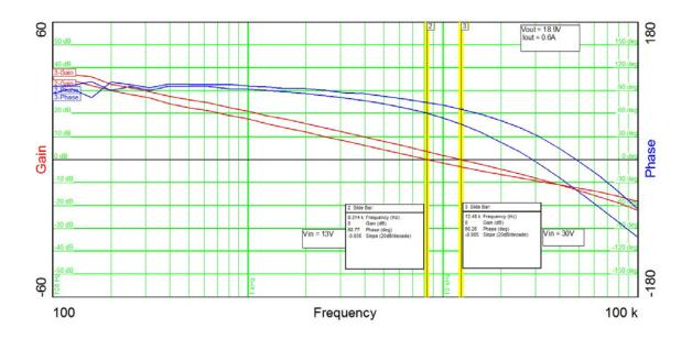
The plot below shows the 18.9V loop gain and phase margin with the output loaded to 0.1A.
