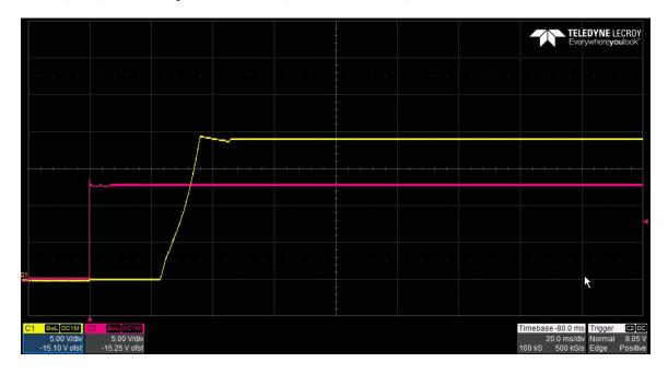
The photo below shows the 18.9V output voltage startup waveform (YELLOW) after the application of 13V in (RED) with the output loaded to 0.6A. (5V/DIV, 20mS/DIV)
