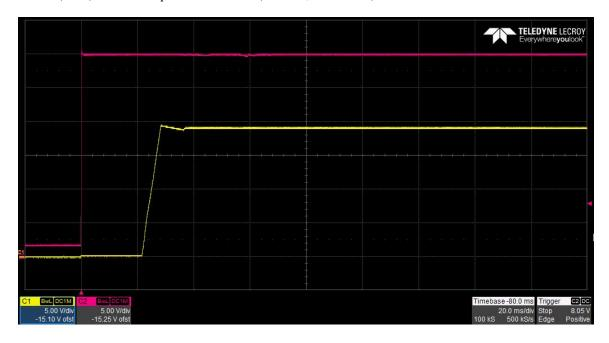
The photo below shows the 18.9V output voltage startup waveform (YELLOW) after the application of 30V in (RED) with the output loaded to 0.6A. (5V/DIV, 20mS/DIV)
