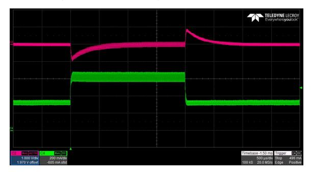
The photo below shows the output voltage (ac coupled) when the load current is stepped between 0.3A and 0.6A. Vin = 30V. (1V/DIV, 200mA/DIV, 500uS/DIV)
