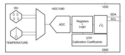
Figure 5. HDC1080 Functional Block Diagram
