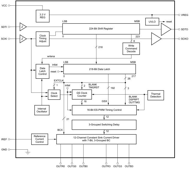
Figure 2. TLC5971 Functional Block Diagram
