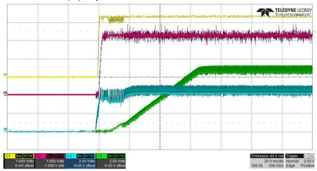
4.6 Start Up @ Vin=692VDC from Line1 to Line2 (692VDC is generated by an AC source with a voltage doubler circuit) input and no load.
