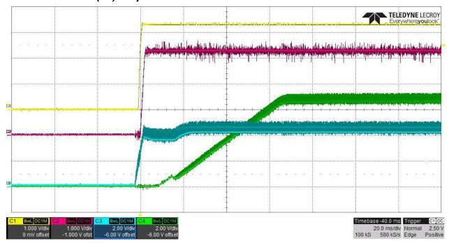
4.4 Start Up @ Vin=340VDC from Line1 to Line2 (340VDC is generated by an AC source with a voltage doubler circuit) input and no load.
