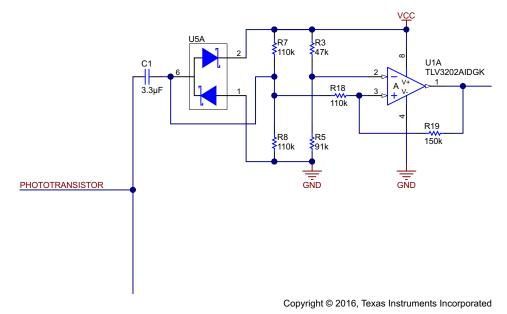
Figure 7. Low to High Transition Logic
