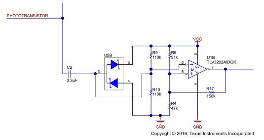
Figure 6. High to Low Transition Logic
