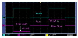
Figure 20. Bidirectional Current Measurements
