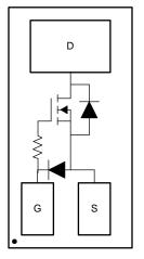
Figure 3. CSD13381F4 Functional Diagram
