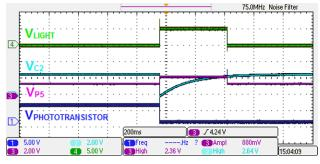
Figure 16. Close IR Filter Pulse Train
