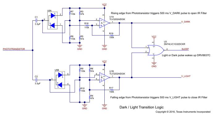
Figure 14. Comparator Pulse Generator
