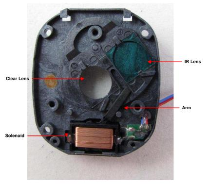
Figure 12. IR Filter Lens and Solenoid
