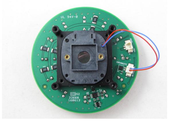
Figure 11. IR Filter Mounted to Backside of PCB
