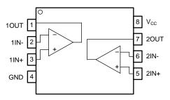
Figure 4. TLV3202AIDGK Functional Diagram
