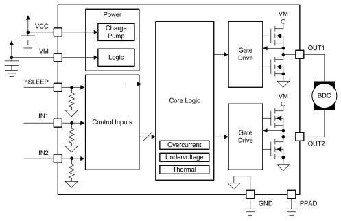
Figure 2. DRV8837C Functional Diagram
