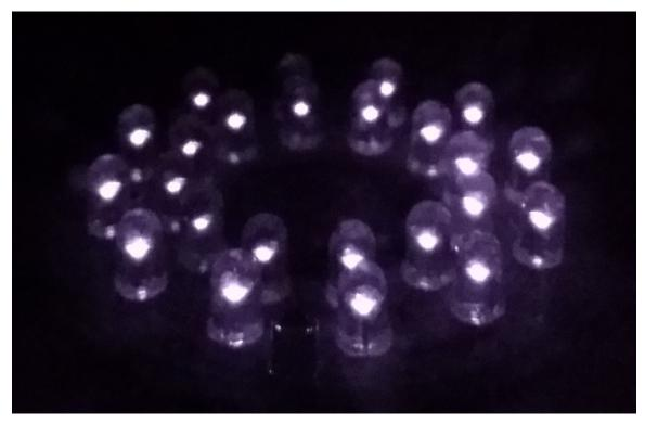
Figure 18. IR LED Illuminated Ring
