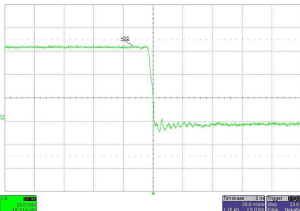
Figure 13.  $V_{DS}$  Turnon Waveform at 48-V Input
