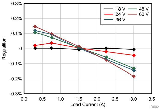
Figure 7. 12-V\_Main Output Voltage Regulation With Load Current
