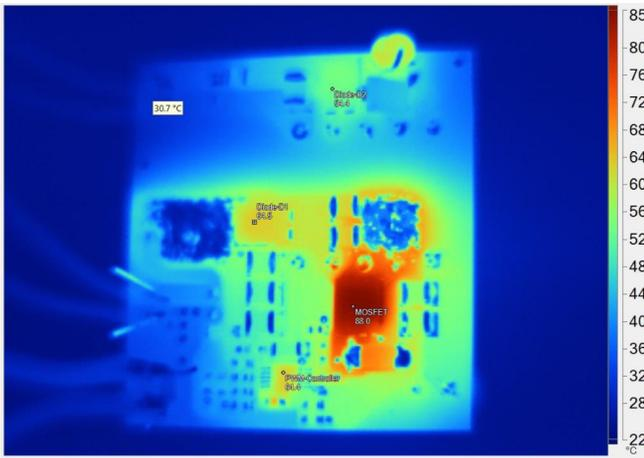
Figure 33. Bottom-Side Thermal Image at 48-V Input, 36 W, and Without Fan
