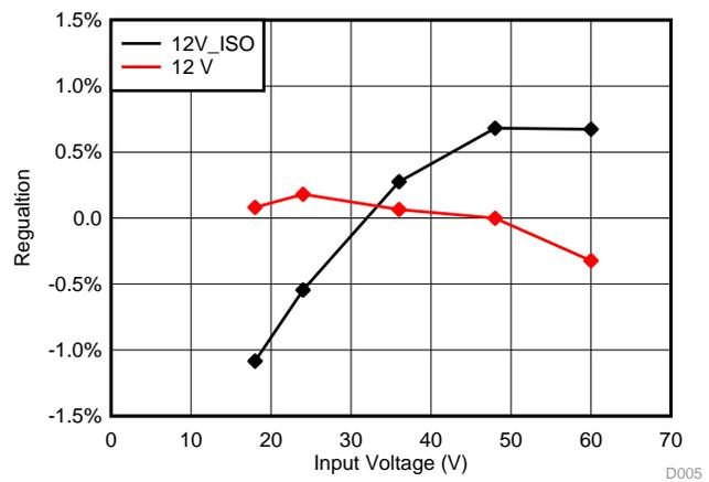
Figure 10. Line Regulation at Full Load
