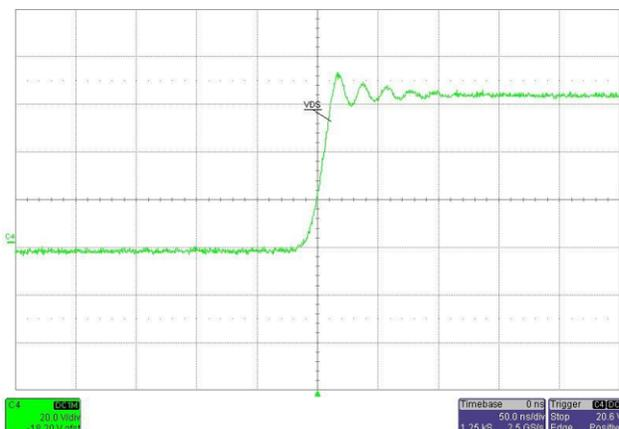
Figure 14.  $V_{DS}$  Turnoff Waveform at 48-V Input
