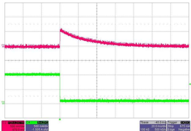
Figure 26. 12-V\_ISO Output Waveform—Load Transient From 1 A to 0.1 A
