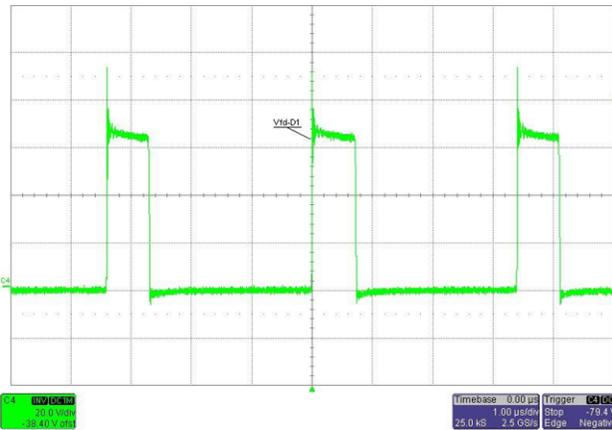
Figure 15. Voltage Across Diode D1 at 48-V Input at Full Load
