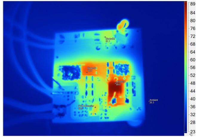
Figure 34. Bottom-Side Thermal Image at 48-V Input, 50 W, and With Fan
