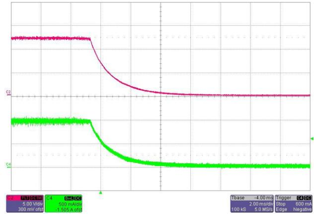
**Figure 22. 12-V\_ISO and 1-A Output Turnoff Waveform at 48 V**
