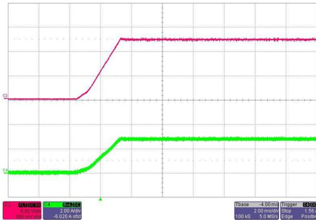
Figure 19. 12-V\_Main and 3-A Output Turnon Waveform at 48 V
