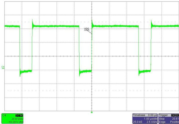
Figure 12. SW Node Waveform  $V_{IN}=48\text{ V}$ , Full Load
