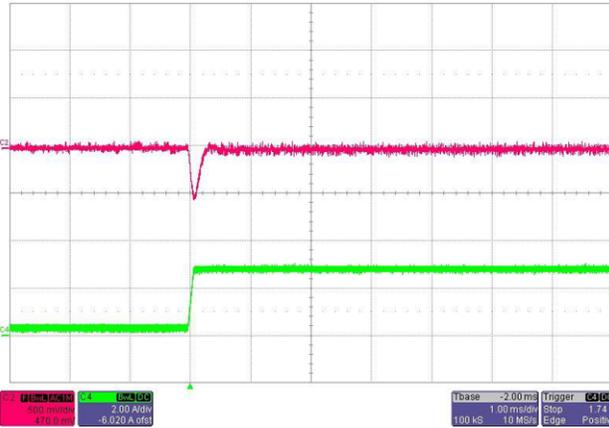
Figure 23. 12-V\_Main Output Waveform—Load Transient From 0.3 A to 3 A
