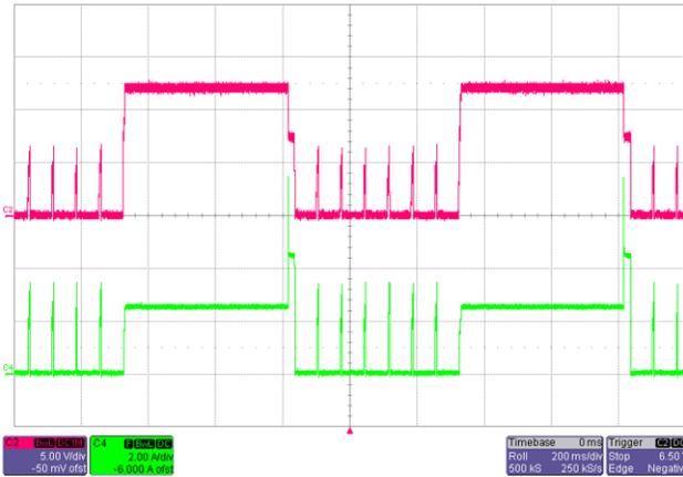
Figure 35. Overcurrent Protection for 12-V Main Output
