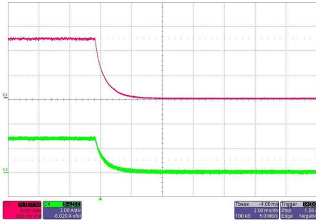
**Figure 21. 12-V\_Main and 3-A Output Turnoff Waveform at 48 V**
