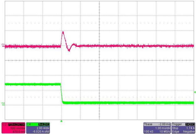
Figure 24. 12-V\_Main Output Waveform—Load Transient From 3 A to 0.3 A
