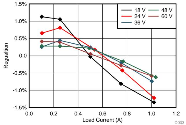
Figure 8. 12-V\_ISO Output Voltage Regulation With Load Current
