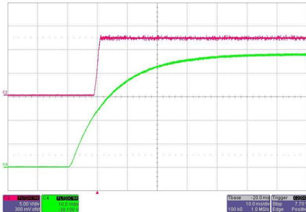
Figure 27. 12-V\_Main Output Waveform—Turnon of Input Voltage
