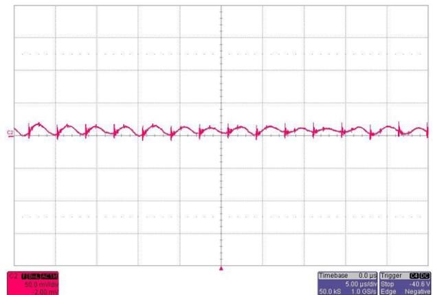
Figure 18. 12-V\_ISO Output Ripple at  $V_{IN}=48\text{ V}$  and Full Load
