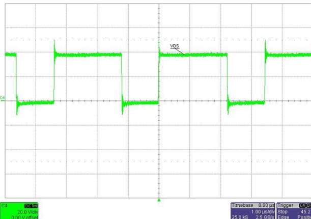
Figure 11. SW Node Waveform  $V_{IN}=24\text{ V}$ , Full Load
