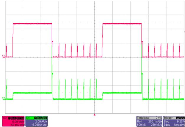
Figure 36. Overcurrent Protection for 12-V Isolated Rail
