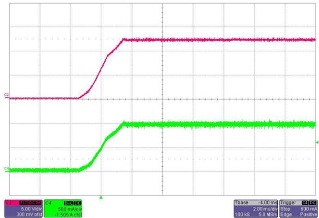
Figure 20. 12-V\_ISO and 1-A Output Turnon Waveform at 48 V
