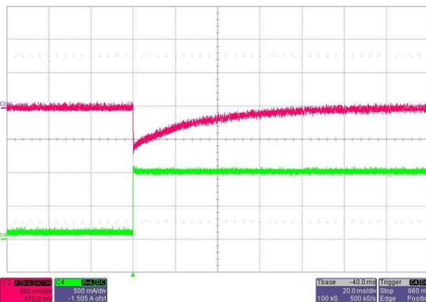
Figure 25. 12-V\_ISO Output Waveform—Load Transient From 0.1 A to 1 A
