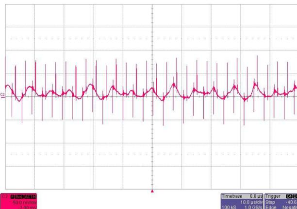
Figure 17. 12-V\_Main Output Ripple at  $V_{IN}=48\text{ V}$  and Full Load
