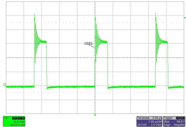
Figure 16. Voltage Across Diode D2 at 48-V Input at Full Load
