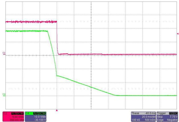
Figure 28. 12-V\_Main Output Waveform—Turnoff of Input Voltage
