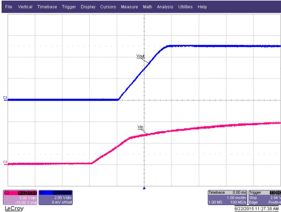
The photo below shows the output voltage startup waveform after the application of 10.8V in with the 5V output loaded to 2A. (Vout: 5V/DIV, 1mS/DIV), (Vin: 2V/DIV)
