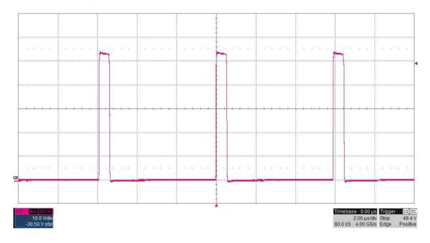
The photo below shows the FET switching voltage (TP2) for an input voltage of 12V and a 1A load. (10V/DIV, 2uS/DIV)
