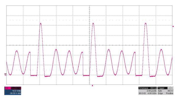
The photo below shows the FET switching voltage (TP2) for an input voltage of 40V and a 0A load. (10V/DIV, 10uS/DIV)
