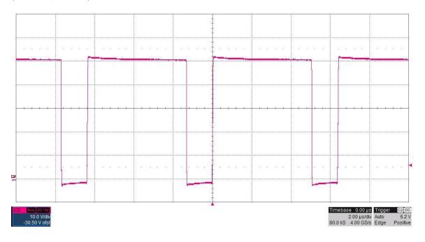
The photo below shows the FET switching voltage (TP2) for an input voltage of 5V and a 0A load. (10V/DIV, 2uS/DIV)
