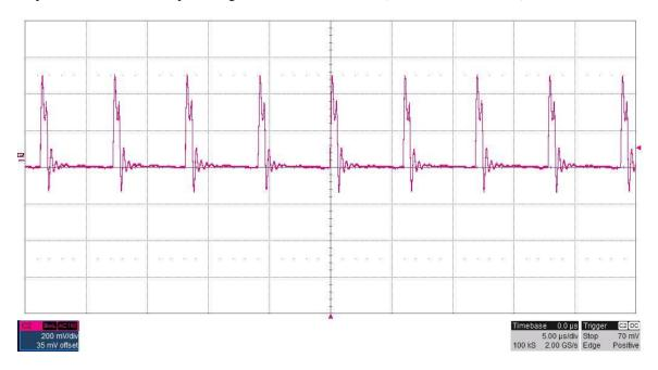
The 50V output ripple voltage (AC coupled) is shown in the figure below. The image was taken with the output loaded to 1A. The input voltage is set to 12V. (100mV/DIV, 5uS/DIV)
