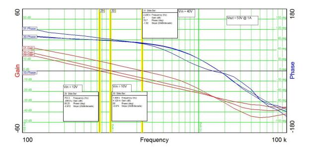
The plot below shows the loop gain at 5V input and the output set to 1A. A 1200uF/63V aluminum capacitor added to the input to reduce the cabling source impedance.
