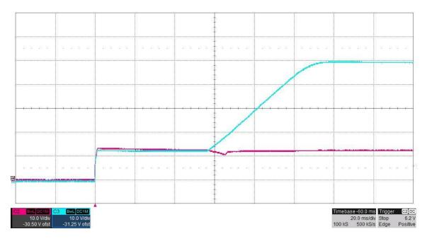
The photo below shows the output voltage startup waveform after the application of 12V in. The 50V output was loaded to 1A. (10V/DIV, 20mS/DIV)
