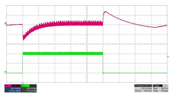
The photo below shows the 50V output voltage (ac coupled) when the load current is stepped between 0.5A and 1A. Vin = 12V. (200mV/DIV, 500mA/DIV, 20mS/DIV)
