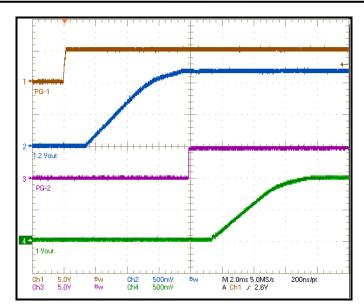
The Shut Down is also sequential. Shut Down of TPS54541 pulls the PG-1 low which causes the Shut Down of TPS56C215 – 1.2 V, 400 kHz converter. The TPS56C215 – 1 V, 1.2 MHz converter follows immediately upon PG-2 going low. Shut Down sequence of converters operating at their full load is shown below.
