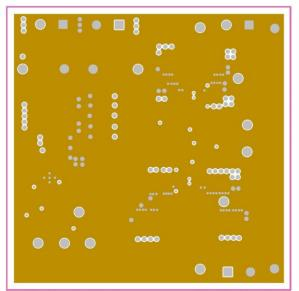
The inner layer-2 is having copper fills of  $V_{IN}$  and  $V_{OUT}$  and is shown below.
