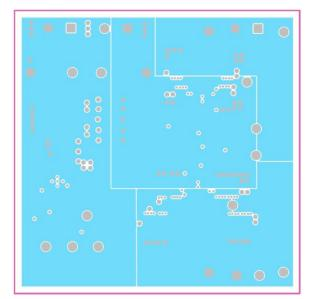
The Bottom Layer is an additional ground plane with output feedbacks, PGOOD and EN signal routings.
