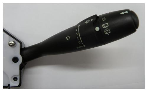
Figure 21. Wiper Control Arm
