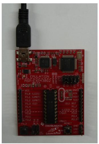
Figure 23. MSP430<sup>™</sup> LaunchPad<sup>™</sup> USB Connection and Jumper Settings
