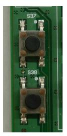
Figure 29. Pushbutton S37 and S38 on IN18
