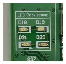
Figure 30. Button and Switch LED Backlighting
