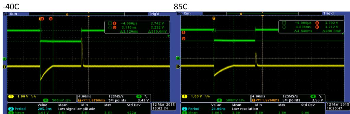
Figure 27. Line Voltage Steps (3.7V to 3.2V), L = 4.7uH, IOU<sub>T</sub> = 40mA
