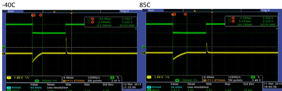
Figure 24. Line Voltage Steps (3.7V to 3.2V), L = 10uH, IOUT = 40mA
