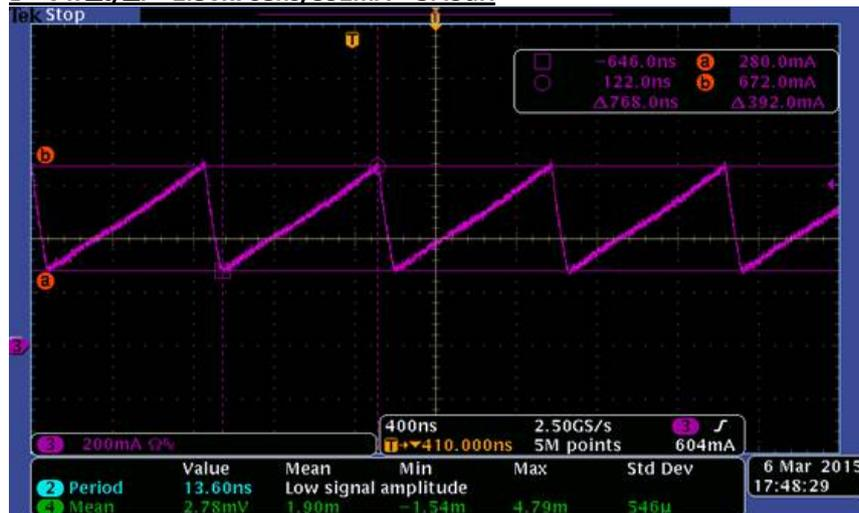
Figure 11. Inductor Current Ripple (2x8 LEDs), L = 4.7μH, TA = 25C, IOU = 40mA
