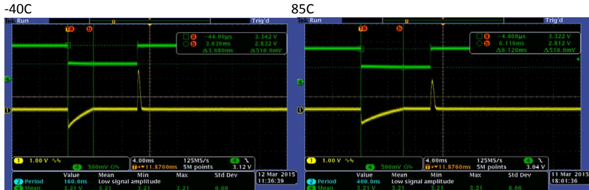
Figure 23. Line Voltage Steps (3.3V to 2.8V), L = 10uH, IOUT = 40mA
