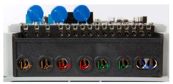
Figure 16. Front View of the EVM With Test Setup Connections
