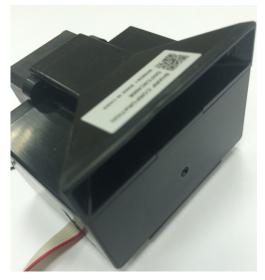
Figure 4. Air Chamber of Sharp DN7C3CA006
