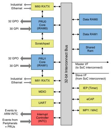
Figure 2. PRU Subsystem Block Diagram
