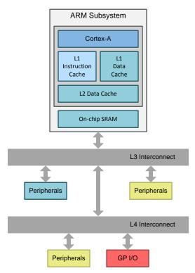
Figure 1. ARM Processor and Interconnects
