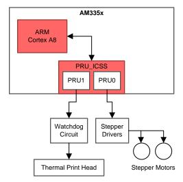
Figure 3. Block Diagram of the Thermal Printer System
