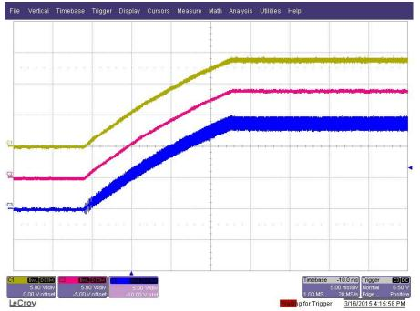
4.1 Start Up @ 110V<sub>DC</sub>: 14V/0.1A, 14V/0.1A, and 14V/0.1A.
