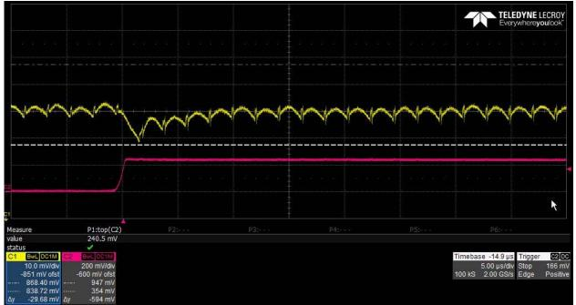
Channel 1 yellow is Vout at output caps and show peak undershoot of 12mV from DC value of Vout Channel 2 is dynamic load current measured as voltage across 30mohms rising from zero mV to 240 mV in 0.8 usec or 0A to 8A at 10A per usec.
