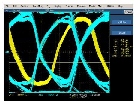
Figure 3 - Measured Setup Time
