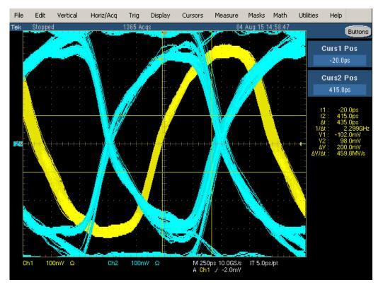
Figure 4 - Measured Hold Time
