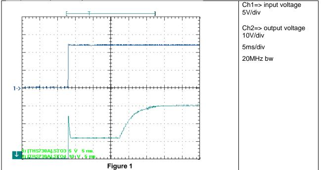
The startup waveform is shown in the Figure 2. The input voltage was set at 12V, with LED load at the output.
