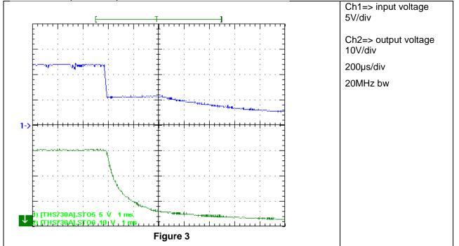
The shutdown waveform is shown in the Figure 4. The input voltage was set at 12V, with LED load on the output. One input cable was disconnected.
