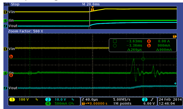
100Vin, 12Vout @ 27.77Ω Load. In-rush zoom.
