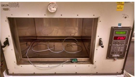
Figure 12: Delta 9064 Environmental Test Chamber and Test Setup
