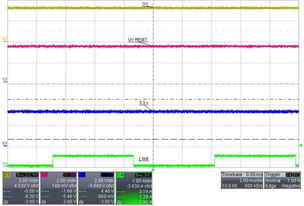
Figure A-3: Load Transient Response - 0 mA to 500 mA on 3.3 V rail
