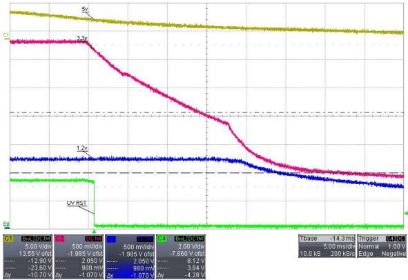
Figure 11: Slow shut down with diode maintaining bias between 3.3 V and 1.2 V rails
