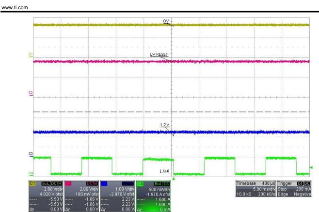
Figure A-7: Load Transient Response - 30 mA to 480 mA on 1.2 V rail
