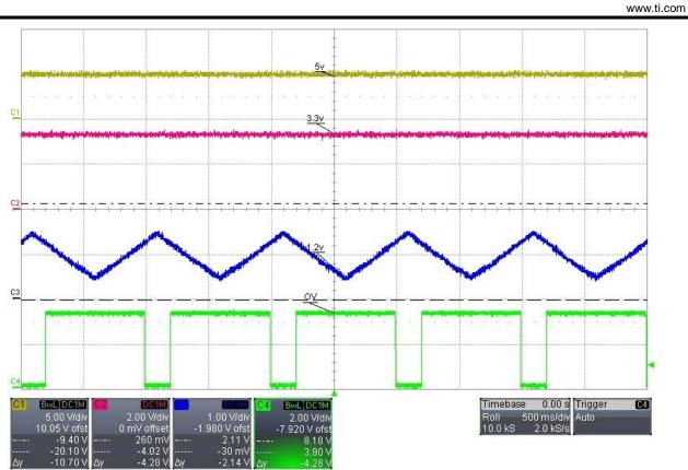
Figure 8: Reset asserted for an overvoltage fault on the 1.2 V rail
