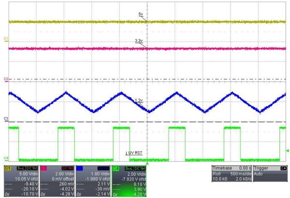
Figure 7: Reset asserted for an undervoltage fault on the 1.2 V rail
