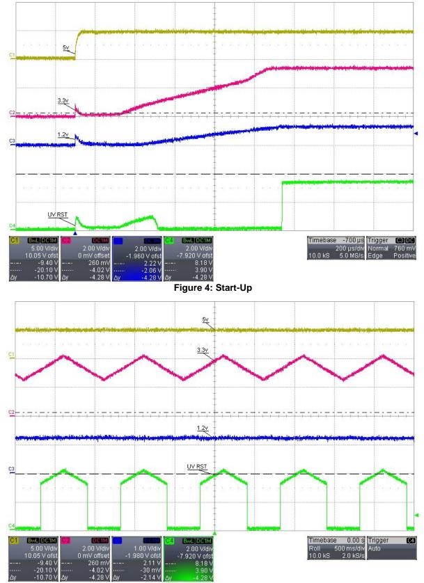
Figure 5: Reset asserted for an undervoltage fault on the 3.3 V rail
