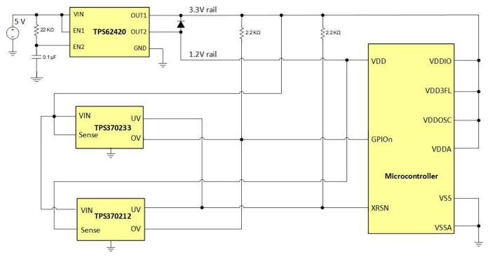
Figure 3: Block diagram showing UV and OV detection
