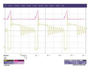
Figure 14 Primary switching voltage and current at 230Vac and full load
