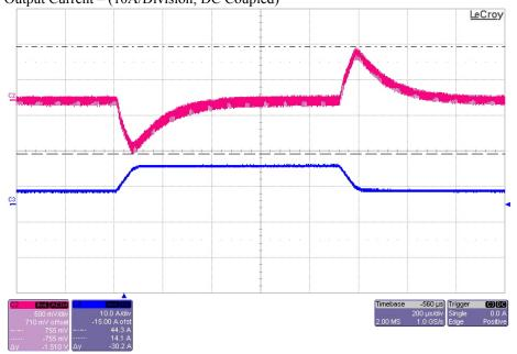
Transient Response – There is a total change of 1.51V to the output voltage
