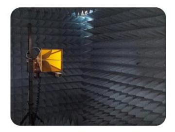
Figure 5: Anechoic Chamber Receive Antenna
