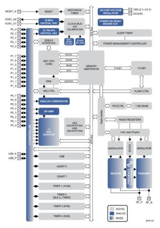
Figure 2: CC2540 Block Diagram
