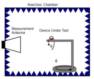
Figure 3: Radiation Pattern Test Setup
