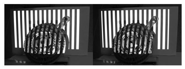
Figure 41 Non-inverted and inverted vertical gray code pattern 6 capture
