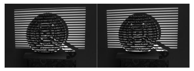
Figure 29 Non-inverted and inverted horizontal gray code pattern 7 capture
