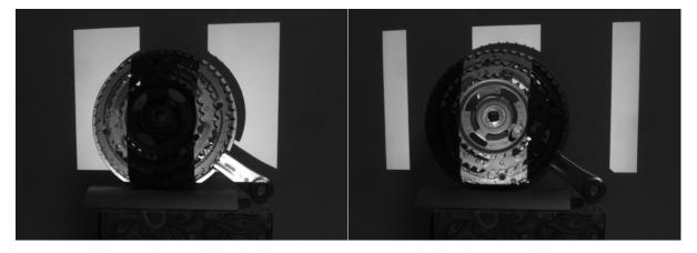
Figure 16 Non-inverted and inverted vertical gray code pattern 3 capture
