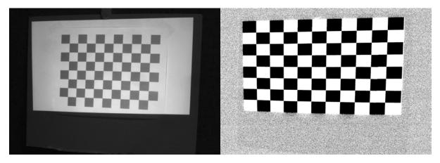
Figure 2 Printed calibration board and projected calibration board position 1
