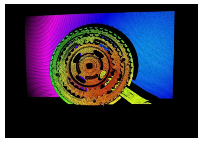
Figure 32 Depth-map of object from 3D scan
