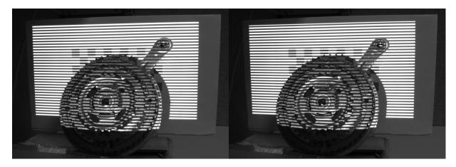
Figure 53 Non-inverted and inverted horizontal gray code pattern 8 capture
