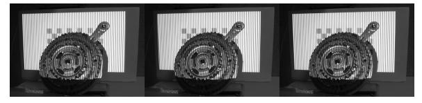
Figure 35 Vertical three phase patterns
