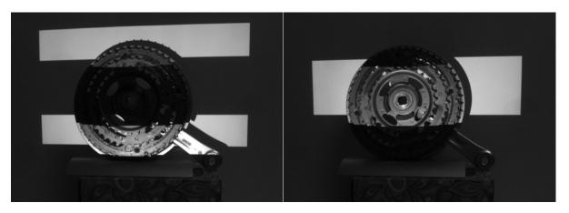
Figure 25 Non-inverted and inverted horizontal gray code pattern 3 capture
