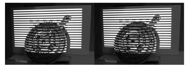
Figure 52 Non-inverted and inverted horizontal gray code pattern 7 capture
