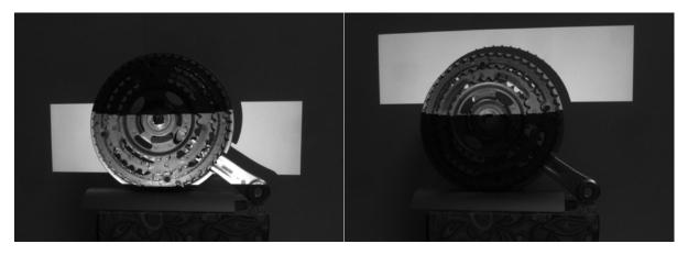
Figure 23 Non-inverted and inverted horizontal gray code pattern 1 capture
