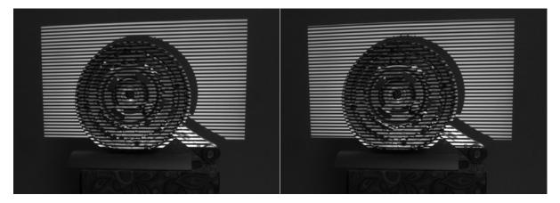
Figure 30 Non-inverted and inverted horizontal gray code pattern 8 capture
