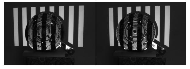
Figure 18 Non-inverted and inverted vertical gray code pattern 5 capture
