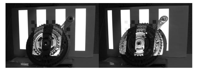
Figure 39 Non-inverted and inverted vertical gray code pattern 4 capture
