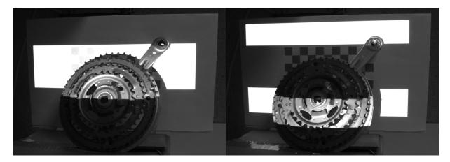
Figure 48 Non-inverted and inverted horizontal gray code pattern 3 capture
