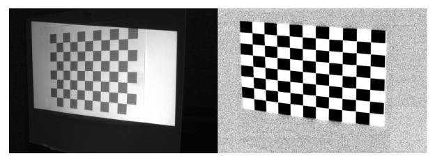
Figure 6 Printed calibration board and projected calibration board position 5
