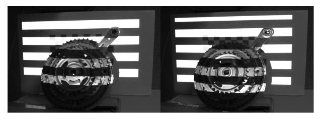
Figure 50 Non-inverted and inverted horizontal gray code pattern 5 capture
