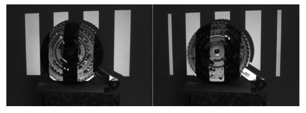
Figure 17 Non-inverted and inverted vertical gray code pattern 4 capture
