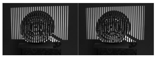
Figure 20 Non-inverted and inverted vertical gray code pattern 7 capture
