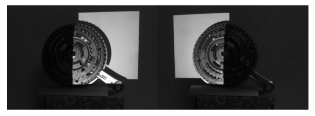
Figure 14 Non-inverted and inverted vertical gray code pattern 1 capture
