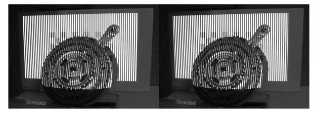
Figure 43 Non-inverted and inverted vertical gray code pattern 8 capture
