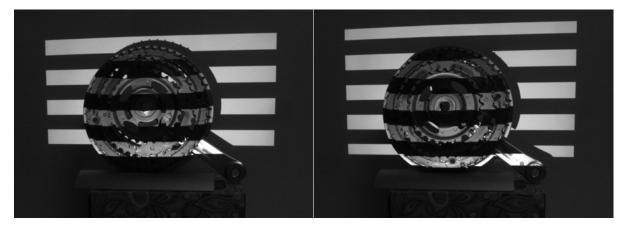
Figure 27 Non-inverted and inverted horizontal gray code pattern 5 capture
