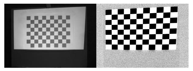
**Figure 11** Printed calibration board and projected calibration board position 10 The following images show examples of the calibration XML files generated for the camera and projector.
