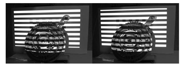
Figure 51 Non-inverted and inverted horizontal gray code pattern 6 capture
