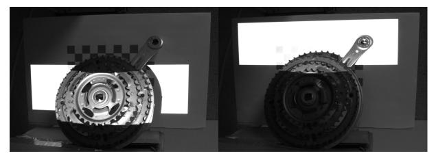
Figure 47 Non-inverted and inverted horizontal gray code pattern 2 capture
