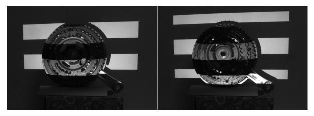
Figure 26 Non-inverted and inverted horizontal gray code pattern 4 capture
