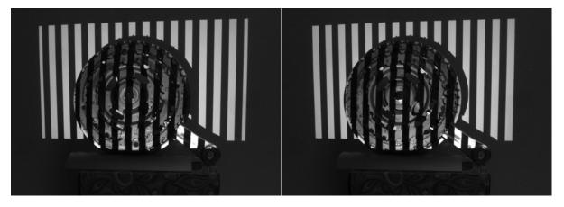
Figure 19 Non-inverted and inverted vertical gray code pattern 6 capture
