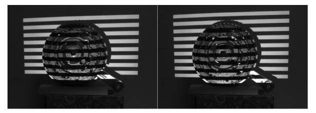
Figure 28 Non-inverted and inverted horizontal gray code pattern 6 capture
