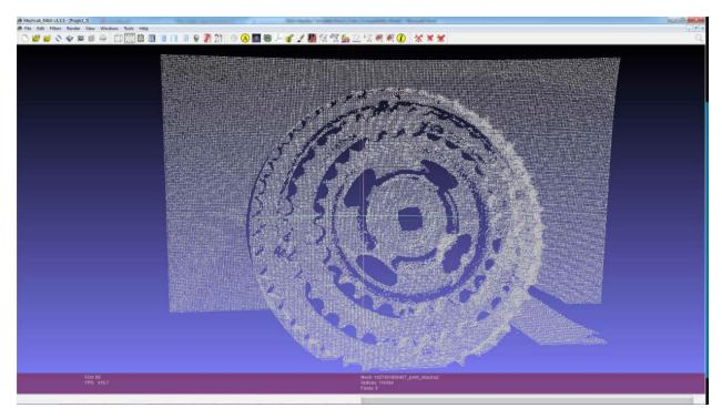
Figure 33 Front view of point-cloud from 3D scan
