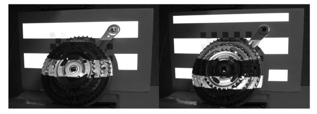
Figure 49 Non-inverted and inverted horizontal gray code pattern 4 capture
