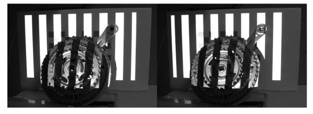
Figure 40 Non-inverted and inverted vertical gray code pattern 5 capture
