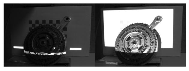
Figure 46 Non-inverted and inverted horizontal gray code pattern 1 capture
