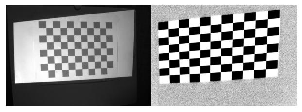
Figure 10 Printed calibration board and projected calibration board position 9
