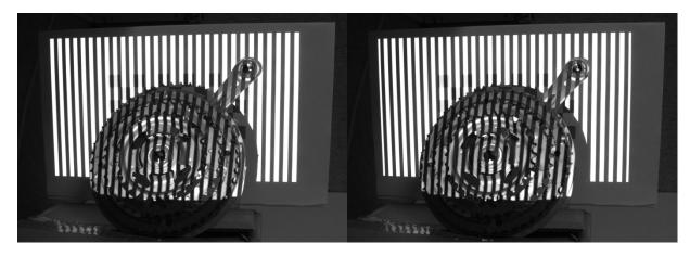
Figure 42 Non-inverted and inverted vertical gray code pattern 7 capture
