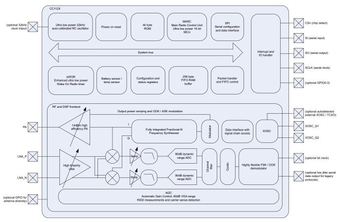
Figure 2. Functional Block Diagram of CC1120
