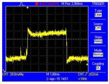
Figure 11. TX Current Plot for One Data Packet in C2OTHER Mode at 869.525 MHz
