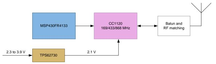
Figure 4. Block Diagram of Multiband wM-Bus RF Subsystem at 169, 433, and 868 MHz
