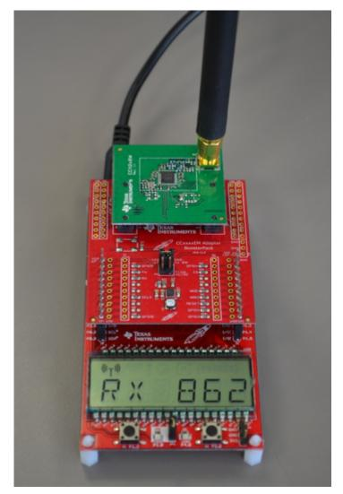
Figure 7. TIDC-Multiband-WMBUS in RX Mode
