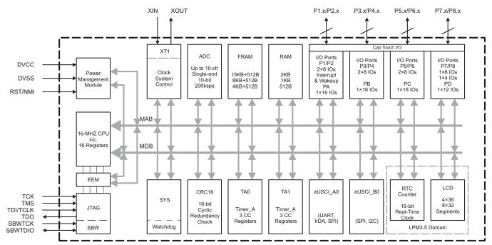
Figure 1. Functional Block Diagram of MSP430FR4133
