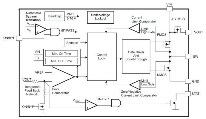
Figure 3. Block Diagram of TPS62730
