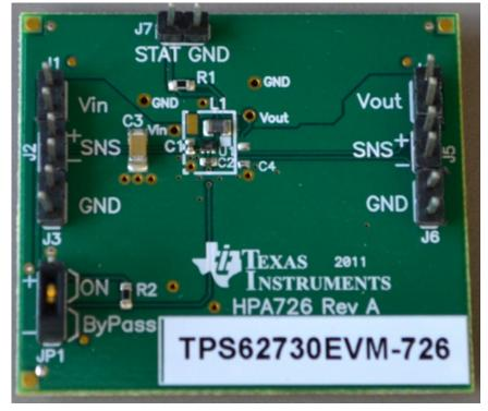
Figure 6. TPS62730 With Jumper Set to ON
