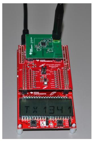
Figure 5. MSP-EXP430FR4133 With TIDC-Multiband-WMBUS (868-MHz Version) and EM Boost Adapter
