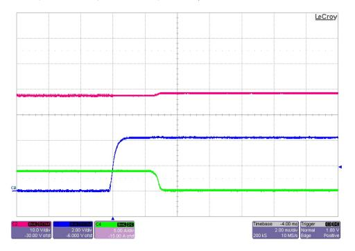
The photo below shows the output current (Green) and DC input voltage (Red) after the ENABLE signal is opened (Blue). The input voltage was set to 38Vdc and the load was 16.5Adc. (Vin is 10V/DIV, EN is 2V/DIV, Iout is 5A/DIV, 2mS/DIV)
