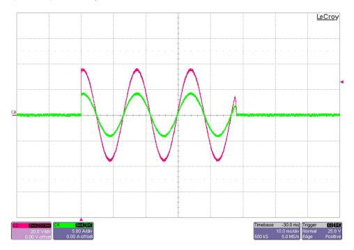
The photo below shows the AC output current (Green) and the output voltage (Red) as the ENABLE signal is transitioned on and off. The input voltage was set to 26Vac and the load was set to 16.5Apk. (20V/DIV, 5A/DIV, 10mS/DIV)
