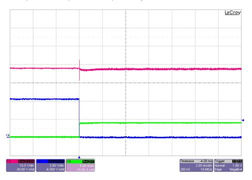
The photo below shows the output current (Green) and DC input voltage (Red) after the ENABLE signal is grounded (Blue). The input voltage was set to 38Vdc and the load was 16.5Adc. (Vin is 10V/DIV, EN is 2V/DIV, Iout is 5A/DIV, 2mS/DIV)
