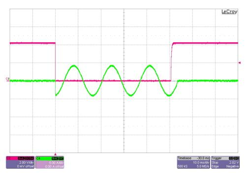
The photo below shows the AC output current (Green) after the ENABLE signal (Red) transitions on and off. The input voltage was set to 26Vac and the load was 3Arms. (2V/DIV, 5A/DIV, 10mS/DIV)
