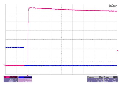
The photo below shows the FET gate-to-source voltage (Red) after the ENABLE signal is opened (Blue). The input bias voltage was set to 12Vdc. (2V/DIV, 1mS/DIV)
