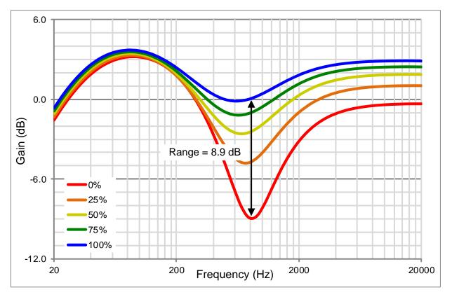
Figure 21: Measured AC Gain Analysis – Mid Control
