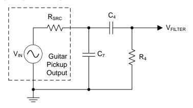
Figure 3: Input Filter Schematic
