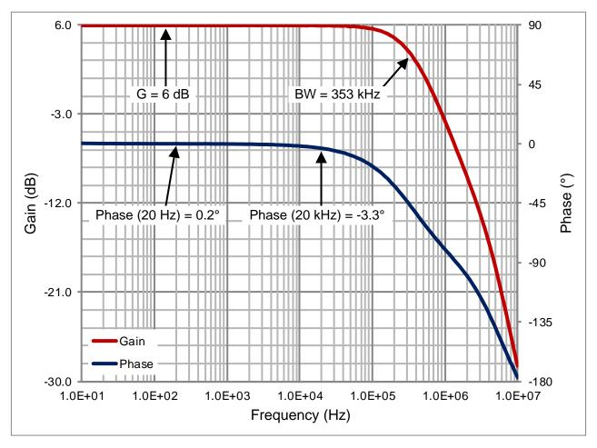
Figure 19: Measured AC Analysis – Input Filter and Gain Stage
