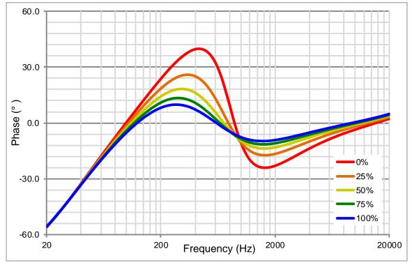
Figure A-3: Measured AC Phase Analysis – Treble Control
