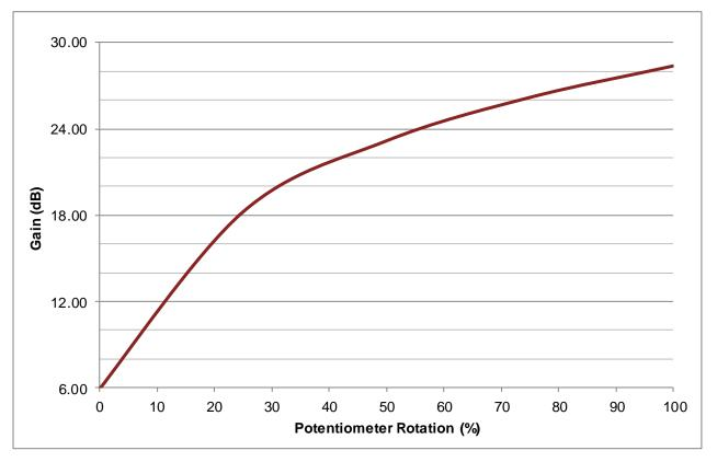
Figure 18: Measured Gain Characteristic
