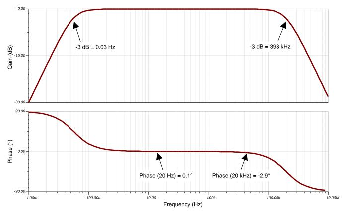
Figure 4: Transfer Function - Input Filter
