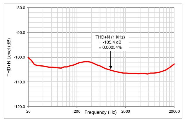
Figure 24: Measured THD+N Level vs. Frequency
