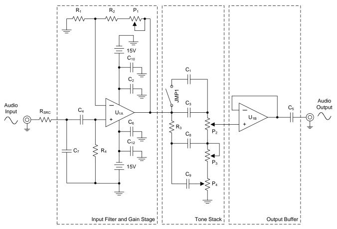
Figure 2: Complete Circuit Schematic
