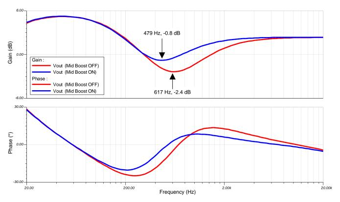
Figure 12: Simulated AC Analysis – Mid Boost
