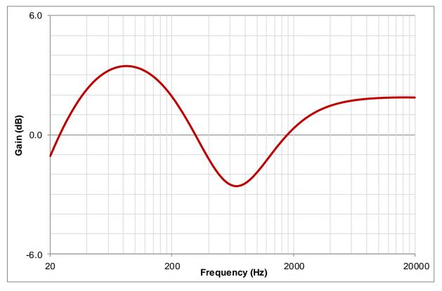
Figure 1: Measured Transfer Function – Bass, Mid, Treble at 50%
