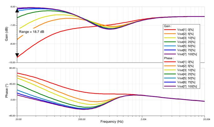
Figure 13: Simulated AC Analysis – Bass Control
