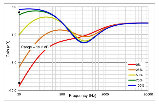
Figure 23: Measured AC Gain Analysis – Bass Control
