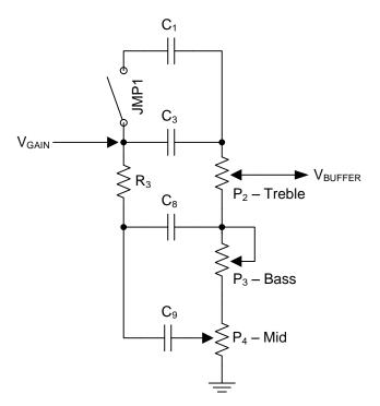
Figure 6: Tone Stack Schematic
