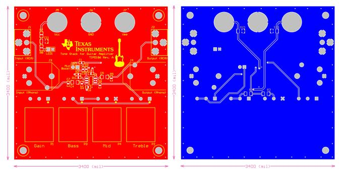
The PCB layout for both layers is shown in Figure 16.
