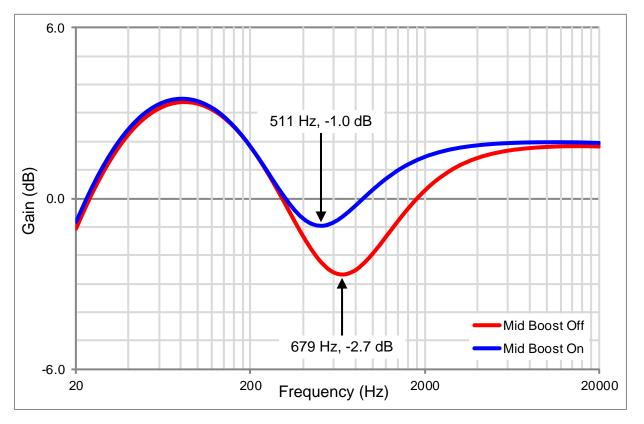
The result of the measured ac gain analysis of the complete circuit as the mid boost jumper is connected and disconnected, when gain = 6dB and all potentiometers are set to 50%, is shown in Figure 22.
