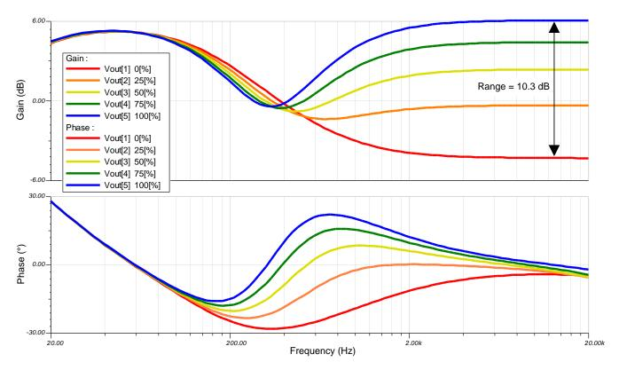
Figure 10: Simulated AC Analysis – Treble Control
