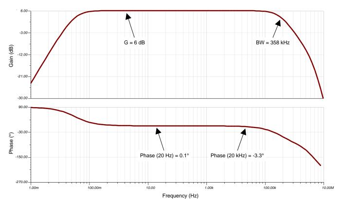
Figure 9: Simulated AC Analysis – Input Filter and Gain Stage
