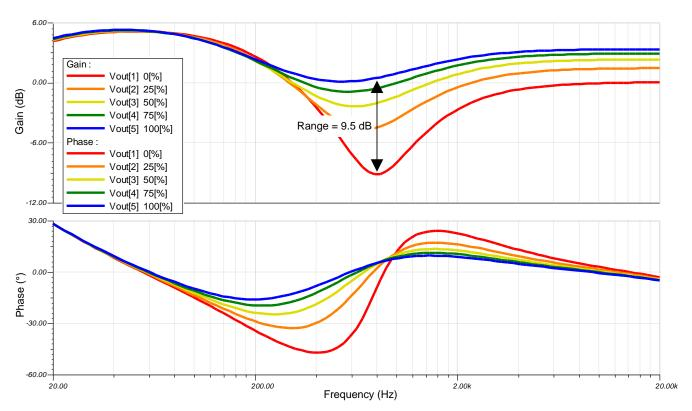
Figure 11: Simulated AC Analysis – Mid Control
