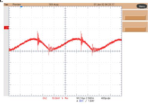
Ch.2: Output Voltage (20mV/div, 40us/div, AC coupling, 20MHz BWL) Iout = 100mA.
