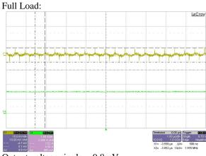
$\overline{\text{Output voltage ripple}} = 9.8 \text{mV}$
