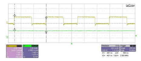
Channel 1 (yellow): SW pin VOUT2 (5V/div) Channel 4 (green): Output Current (1A/div)
