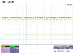
Output voltage ripple = 7.2mV
