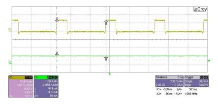
Channel 1 (yellow): SW pin VOUT3 (5V/div) Channel 4 (green): Output Current (500mA/div)
