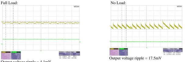
Output voltage ripple = 4.1 mV
