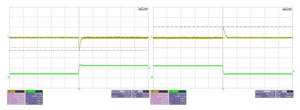
Channel 1 (yellow): VOUT2 Output (10mV/div) Channel 4 (green): Output Current (1A/div) Slewed from 0.2A - 0.8A
