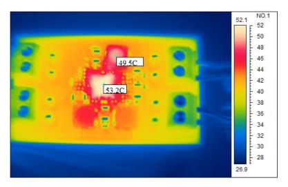
Front Side – Max Temp =  $53.2^{\circ}$ C
