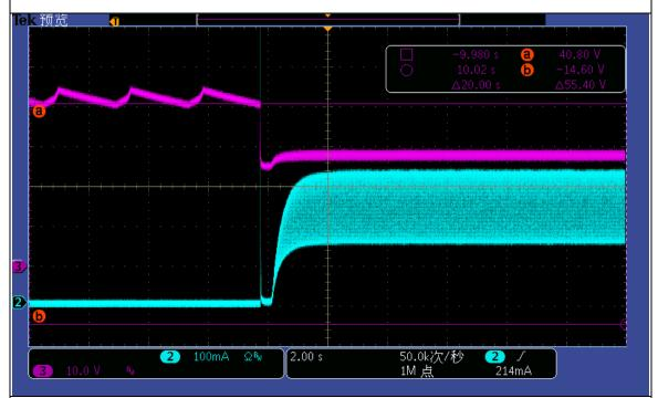
Vin:230Vac From no load to full load
