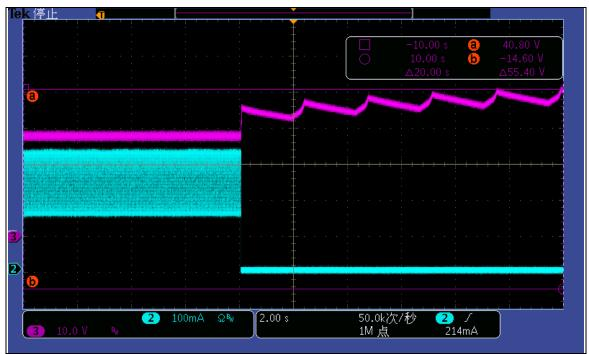
Vin:110Vac From full load to no load
