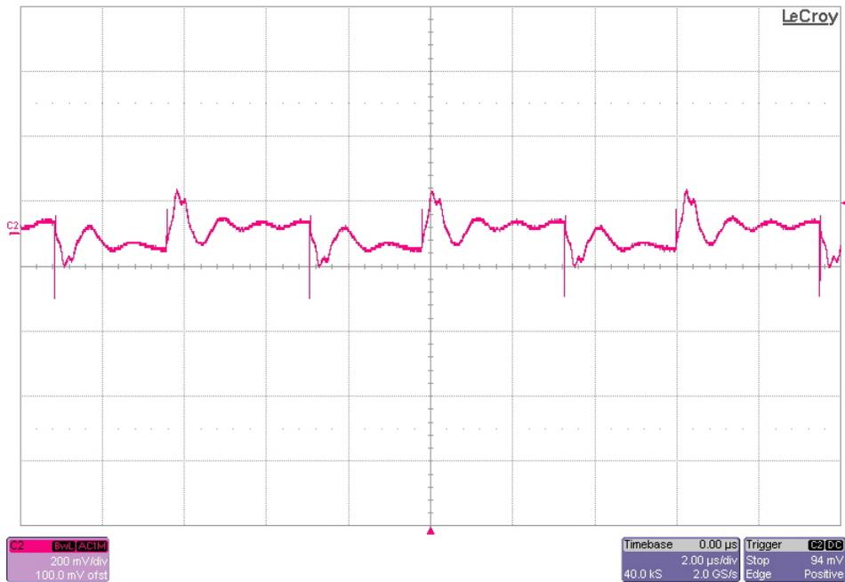
The 12V output ripple voltage (AC coupled) is shown in the figure below. The image was taken with the output loaded to 5A. The input voltage is set to 12V. (200mV/DIV, 2uS/DIV)
