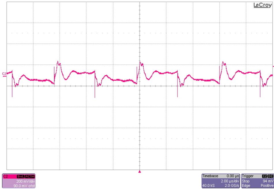
The 12V output ripple voltage (AC coupled) is shown in the figure below. The image was taken with the output loaded to 1A. The input voltage is set to 12V. (50mV/DIV, 2uS/DIV)
