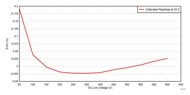
Figure 44. DC Link Voltage versus Error
