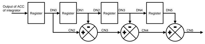
Figure 17. Sinc3 Filter Differentiation Implementation in PRU
