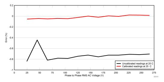
Figure 41. Phase-to-Phase Voltage versus Error
