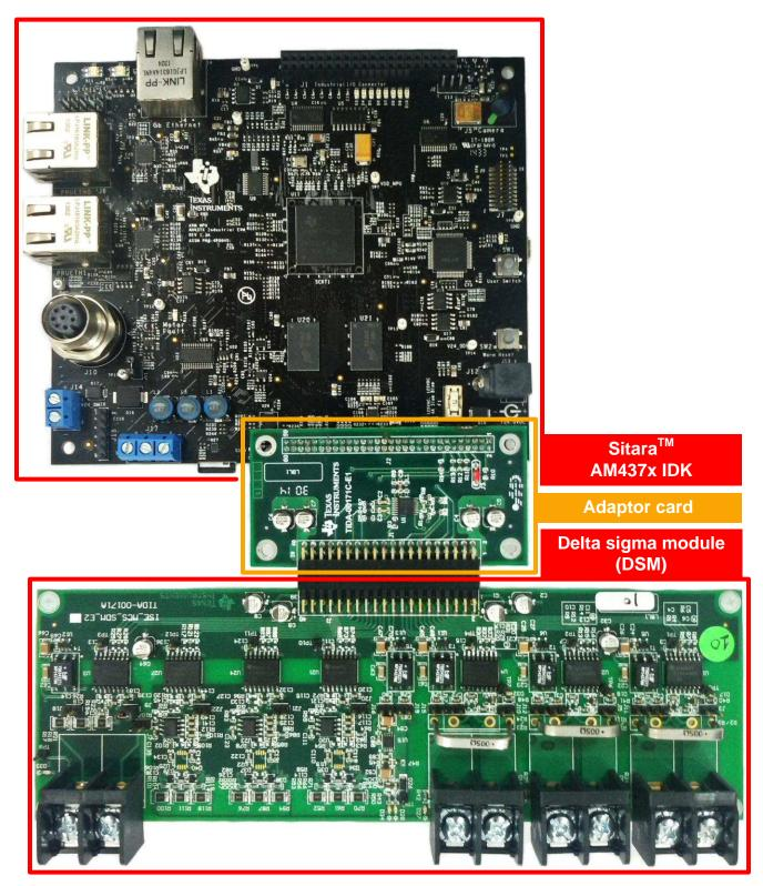
Figure 5. Picture of Isolated Current and Voltage Measurement Kit
