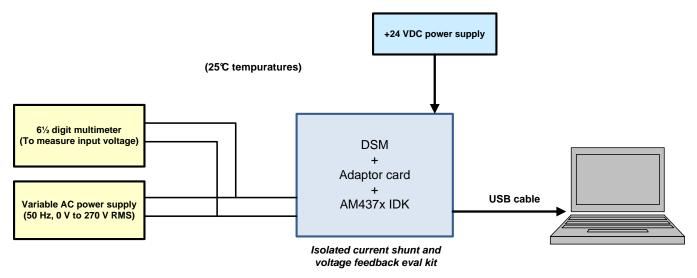
Figure 40. Test Setup for AC Voltage Measurement Accuracy
