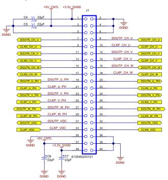
Figure 11. 2×10 Connector Interface With DSM Board
