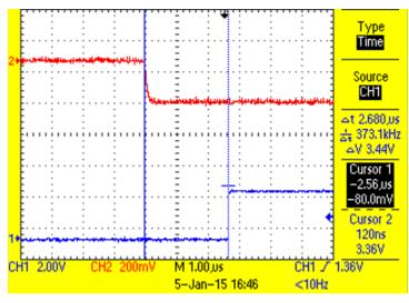
Figure 49. Short Circuit Signal Applied to AMC1304 (Red) and Signal From AM437x (Blue)
