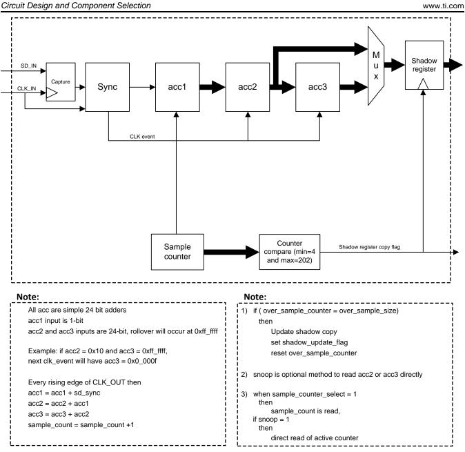
Figure 15. Integrator Block Diagram in ICSS-PRU
