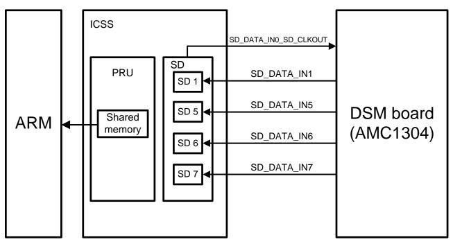
Figure 18. Application Interface With PRU Sigma-Delta Firmware
