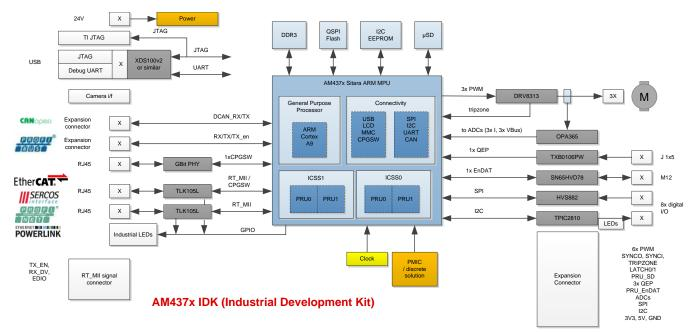
Figure 8. Block Diagram of AM437x IDK
