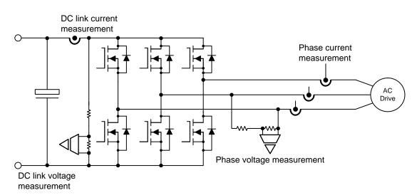
Figure 1. Current and Voltage Measurements in Three-Phase Inverters
