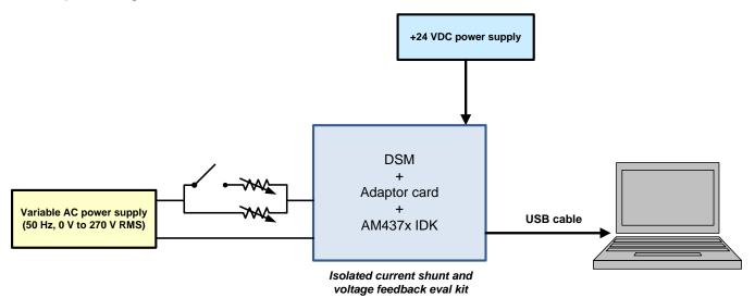
Figure 47. Test Setup for Short Circuit Testing
