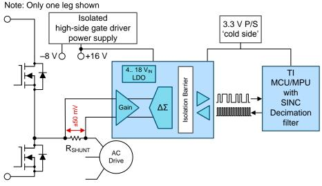
Figure 2. Delta-Sigma Modulator in Three-Phase Inverters
