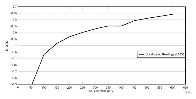
Figure 43. DC Link Voltage versus Error, Uncalibrated Readings at 25°C
