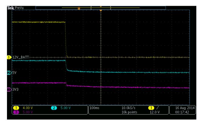
Figure 2 – Shut-down sequence
