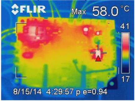
Figure 12 – PCB thermal image @ 20V
