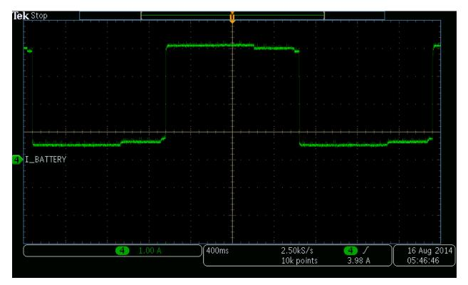
Figure 3 – System current consumption
