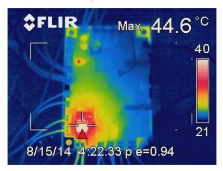
Figure 11 – PCB thermal image @ 12V
