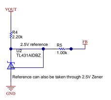
This gives around 0.8V reference to FB (R1 and R5 potential divider) and for locking the feedback the rest 0.2V comes from the Drop across Current Sense resistor and hence can be changes accordingly.
