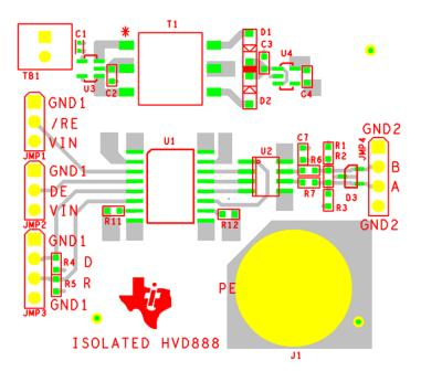
Figure 6: PCB layout top
