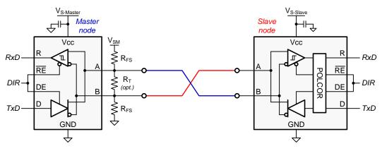
Figure 1: Point-to-point data link with cross-wire fault
