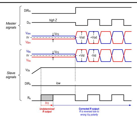
Figure 2: Polarity correcting timing prior to data transmission
