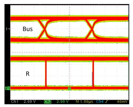
Figure 4: Eye diagram - 250kbps at 300m
