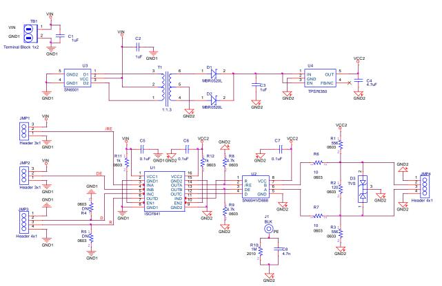
Figure 10: Isolated auto-polarity RS-485 transceiver schematic
