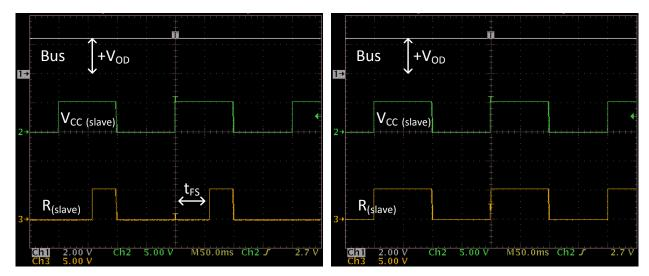
Figure 5: Polarity correction with (left) and without (right) cross-wire fault
