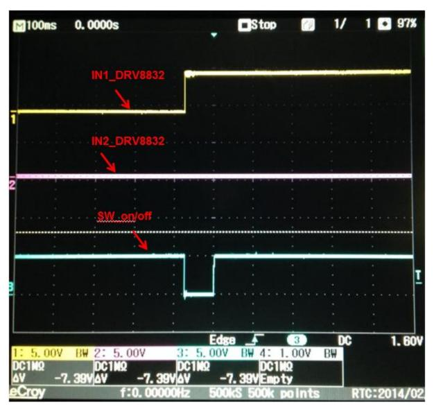
In the above figure, the signals illustrate the situation when the flip up display is commanded to CLOSE. The user switch (SW\_on/off) is pressed, IN1 is high, IN2 is low, and the flip up display closes. The oscilloscope is set to trigger off of the user switch (SW\_on/off).
