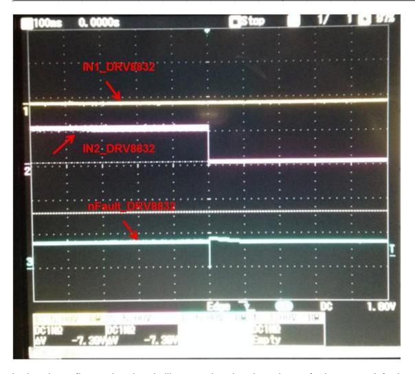
In the above figure, the signals illustrate the situation when a fault occurs. A fault occurs when an overcurrent is reached. In this case, an obstacle (the user's hand) was put in front of the display as it was moving. The flip up display was opening (IN1=0, IN2=1), a fault occurred, then the display stopped moving (IN1=0, IN2=0). The oscilloscope is set to trigger off of the nFault signal.
