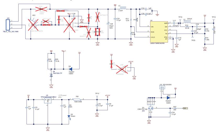
Figure 21. TIDA-00191 Schematic Page 3 (LM5017)
