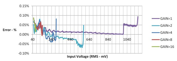
Figure 20. PGA116 Gain Error Over Input Range (25°C)
