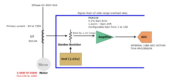
Figure 3. PGA116 Configuration in TIDA-00191
