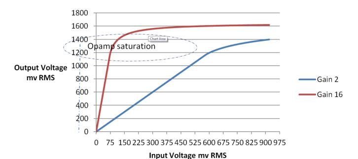
Figure 15. PGA116 Saturation for TIDA-00191
