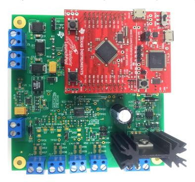
Figure 1. Analog Front End for Motor Electronic Overload Relays with Enhanced Current Range
