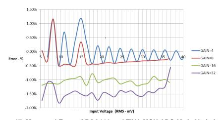
Figure 17. Measured Error of PGA116 and TIVA MCU ADC (Gain Variations)
