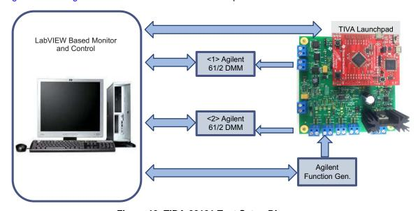
Figure 13. TIDA-00191 Test Setup Diagram
