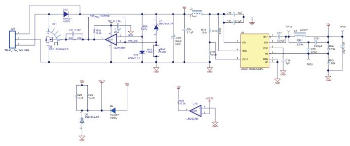
Figure 10. Self-Power Supply Using LM5017
