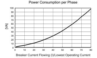
Figure 11. Typical Power Consumption for Current or Lowest Operating Current
