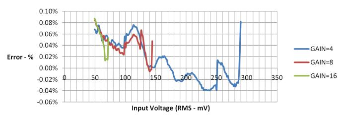
Figure 19. PGA116 Gain Error over Input Range (25°C)
