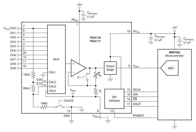
Figure 4. PGA116 Interface to MCU - Block Diagram
