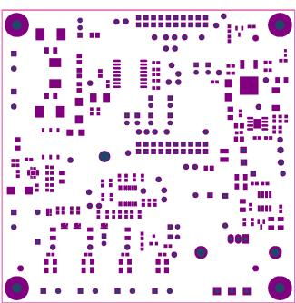
Figure 27. TIDA-00191 — Top Solder Mask
