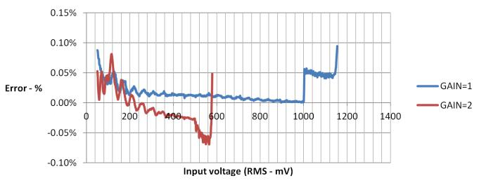
Figure 18. PGA116 Gain Error over Input Range (25°C)
