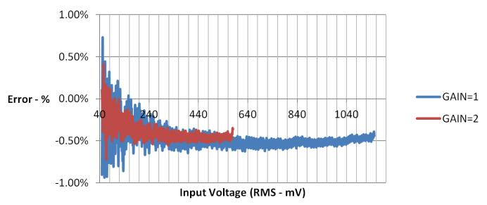
Figure 16. Measured Error of PGA116 and TIVA MCU ADC
