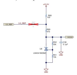
Figure 5. Voltage Reference for Level Shifting
