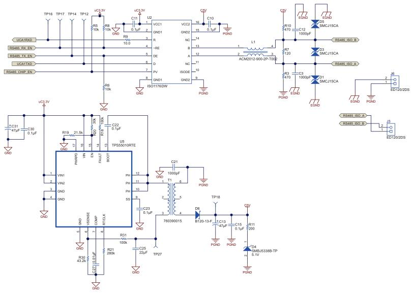
Figure 23. TIDA-00191 Schematic Page 5 (TPS5501 + ISO1176)
