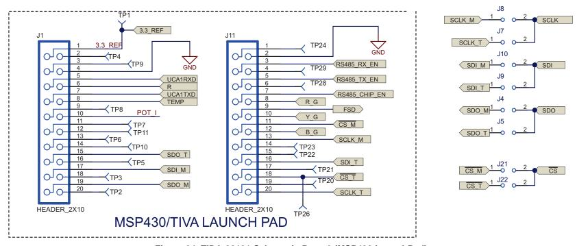
Figure 24. TIDA-00191 Schematic Page 6 (MSP430 LaunchPad)
