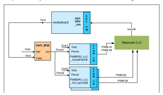
Figure 14. Build Level 3 Block Diagram
