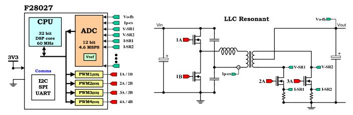
Figure 1. TMDSHVRESLLCKIT Circuit Diagram
