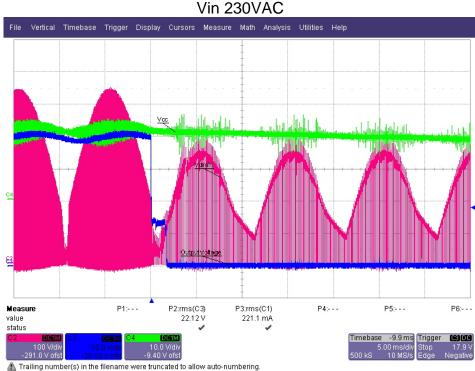
When a short circuit condition occurs, the controller goes into a hiccup mode and reverts back once the short condition is removed.
