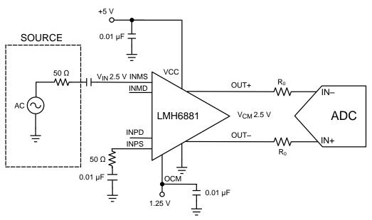
Figure 1. Single-Ended Input With Differential Output
