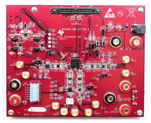
Figure 7. LMH6881 and ADS4449 Test Board
