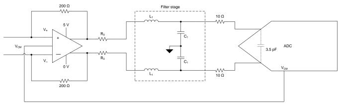
Figure 6. Typical Interface Circuit Driving an ADC
