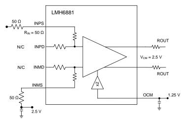
Figure 2. DC-Coupled Configuration
