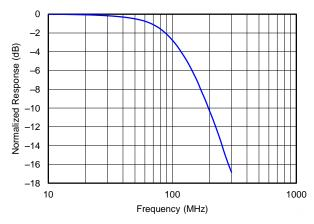
Figure 11. Normalized Gain Response — AC-Coupled
