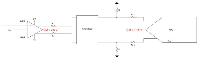
Figure 4. Interfacing With DC-Coupled Configuration
