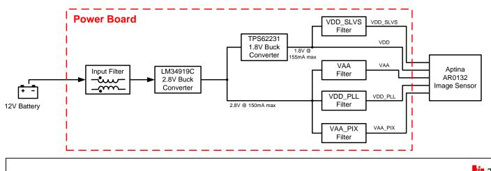
**PMP9300** is designed to power the Aptina AR0132 image sensor in automotive camera applications. The power board provides 1.8V and 2.8V outputs to cover the core, analog and I/O supply required by the sensor IC. The filter board make the design support transferring power and FPD-Link III signals over coax cable configuration.
