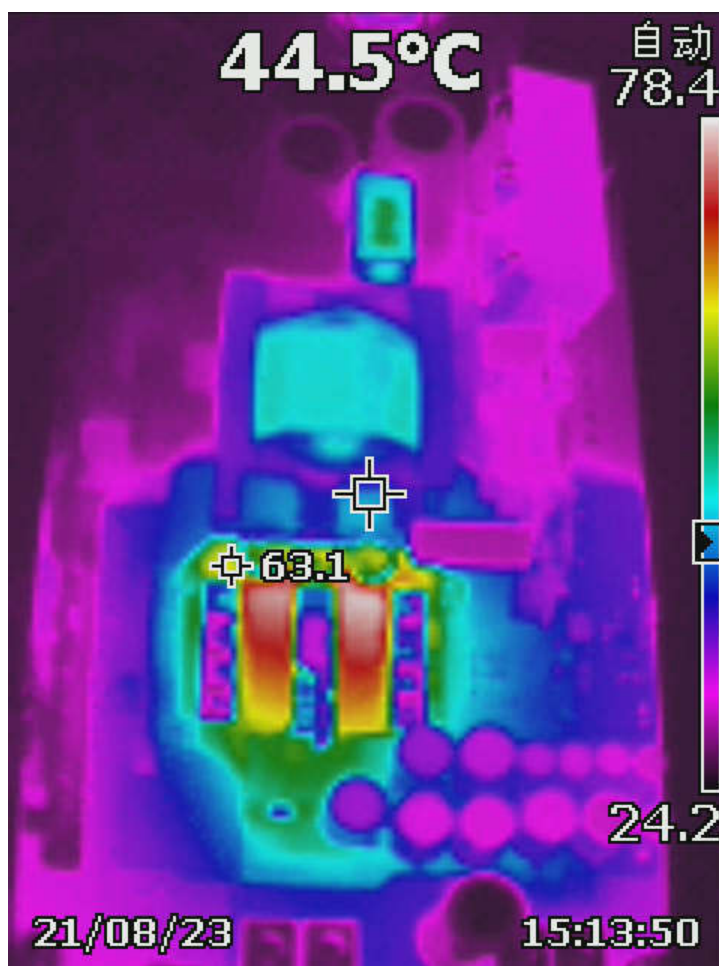
Figure 2-4. Thermal Image: 400-VDC Input With 84-A Load
