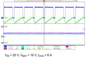
Figure 3-5. Typical PWM Charge Waveform
