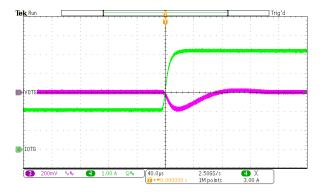
$$\begin{split} V_{BAT} &= 10 \text{ V}, \text{ } V_{OTG} = 5 \text{ V}, \\ I_{OTG} &= 2 \text{ A to } 5 \text{ A}, \text{ } C_{OTG} = 10 \text{ } \mu\text{F} \times 6 + 33 \text{ } \mu\text{F} + 100 \text{ } \mu\text{F} \\ \textbf{Figure 3-9. OTG Transient (Rising Edge)} \end{split}$$
