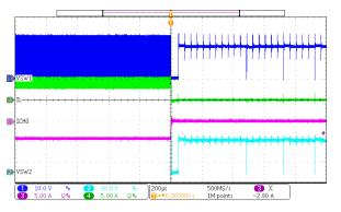
$V_{IN}$  = 20 V,  $V_{BAT}$  = 16 V,  $V_{SYS}$  = 16.3 V,  $I_{CHG}$  = 4 A Figure 3-4. Charge Disable
