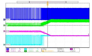
$V_{\text{IN}} = 20 \text{ V}, V_{\text{BAT}} = 16 \text{ V}, V_{\text{SYS}} = 16.3 \text{ V}, I_{\text{CHG}} = 4 \text{ A}$ Figure 3-3. Charge Enable
