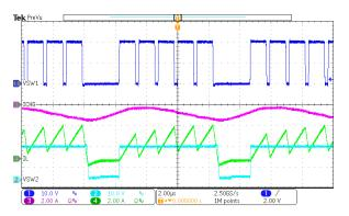
$V_{IN}$  = 20 V,  $V_{BAT}$  = 16 V,  $I_{CHG}$  = 1 A Figure 3-6. Typical PFM Charge Waveform
