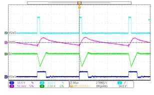
V<sub>BAT</sub> = 16 V, V<sub>OTG</sub> = 5 V, I<sub>OTG</sub> = 200 mA Figure 3-8. Typical PFM OTG Waveform
