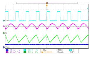
V<sub>BAT</sub> = 16 V, V<sub>OTG</sub> = 5 V, I<sub>OTG</sub> = 2 A Figure 3-7. Typical PWM OTG Waveform
