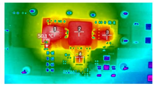
Q1 FET temperature = 48.6°C, IND temperature = 46.8°C Q4 FET temperature = 46.3°C, IC temperature = 45.8°C
