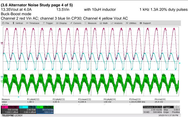
Input ripple 1kHz 1.8Vp-p output 1 kHz ripple (not including switching frequency ripple) 80mVp-p or 27dB attenuation
