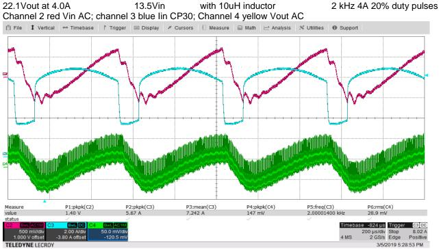
Input ripple 2kHz 1.25Vp-p output 2 kHz ripple (not including switching frequency ripple) 70mVp-p or 25dB attenuation
