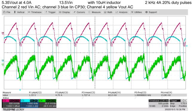
Input ripple 2kHz 1.25Vp-p output 2 kHz ripple (not including switching frequency ripple) 45mVp-p or 29dB attenuation
