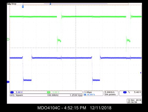
Boost mode: 30V, 10A, Boost Switch Node 30ns of jitter
