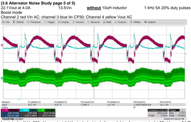
Input ripple 1kHz 530mVp-p output 1 kHz ripple (not including switching frequency ripple) 35mVp-p or 24dB attenuation
