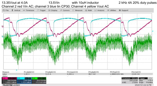
Input ripple 2kHz 1.2Vp-p output 2 kHz ripple (not including switching frequency ripple) 55mVp-p or 27dB attenuation
