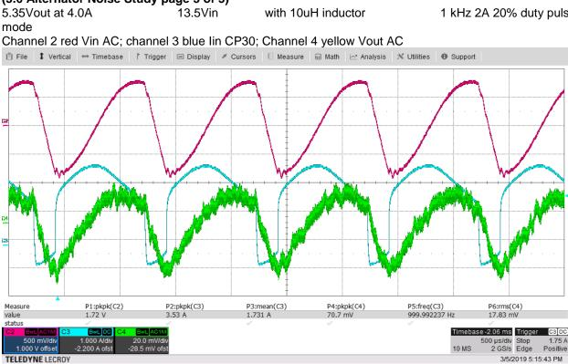
Input ripple 1kHz 1.7Vp-p output 1 kHz ripple (not including switching frequency ripple) 60mVp-p or 29dB attenuation
