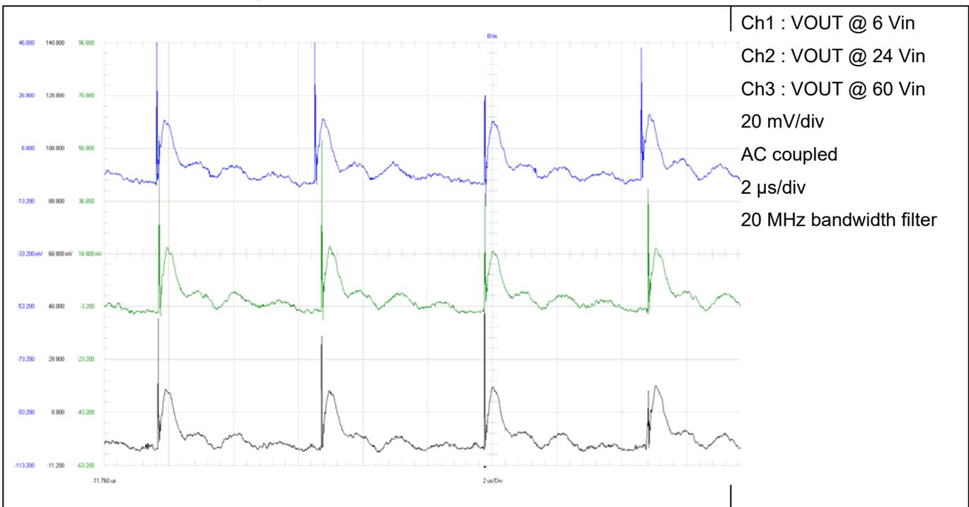
Figure 23. 11 V Output Voltage (Non-isolated)
