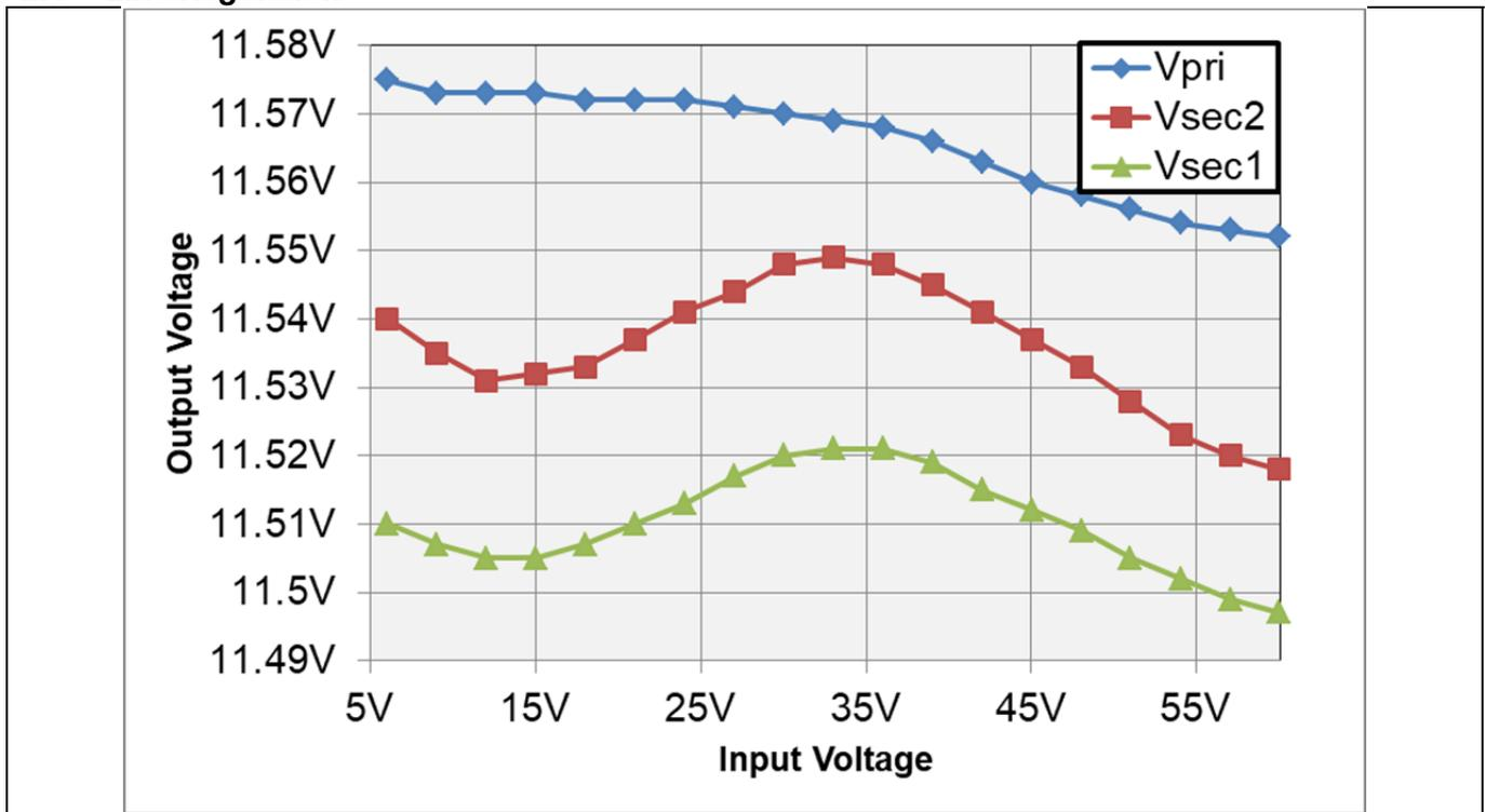
Figure 9. Output Voltage vs Input Voltage for the 11 V Outputs
