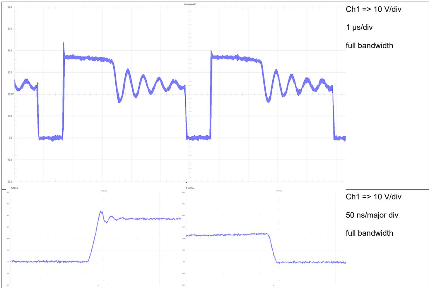
Figure 16. Switchnode to GND @ 24 Vin
