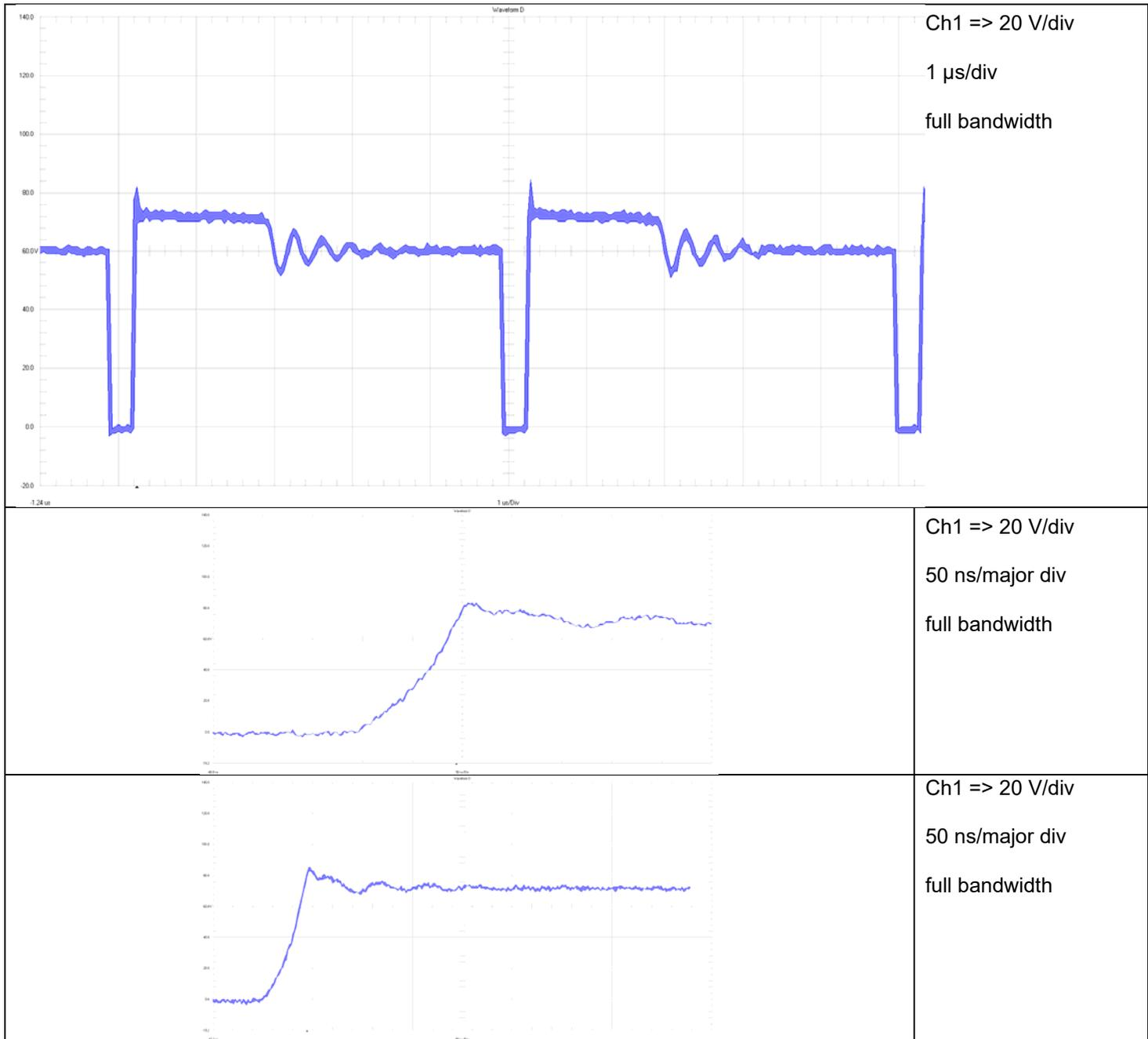
Figure 18 Switchnode to GND @ 60 Vin Flyback with R200 =10 kOhms
