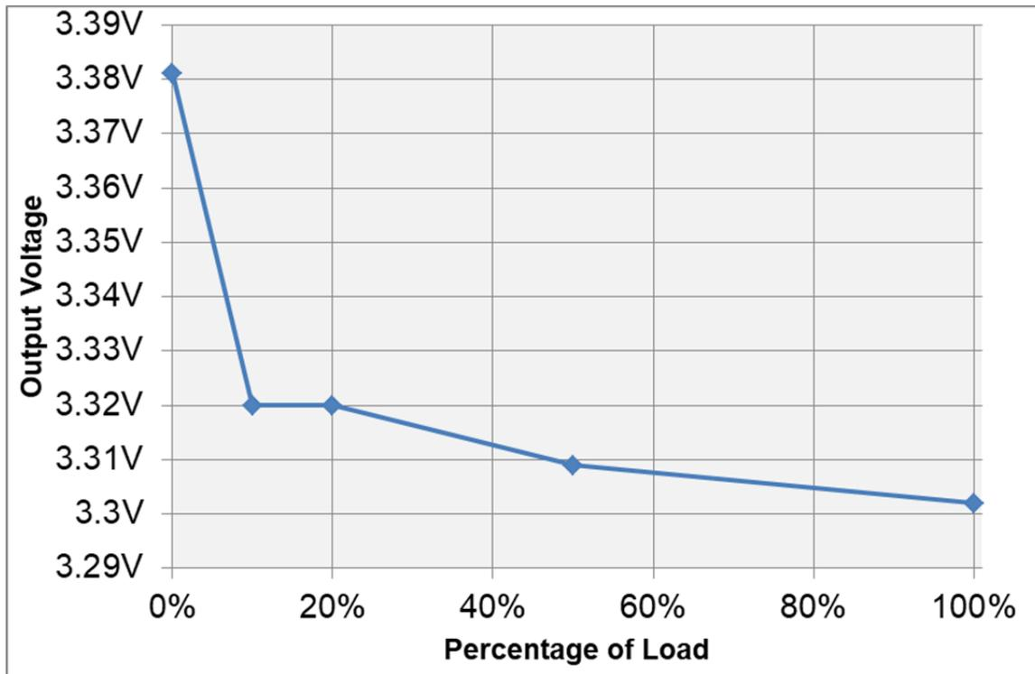
Figure 8. Output Voltage vs Load for the 3.3 V Output
