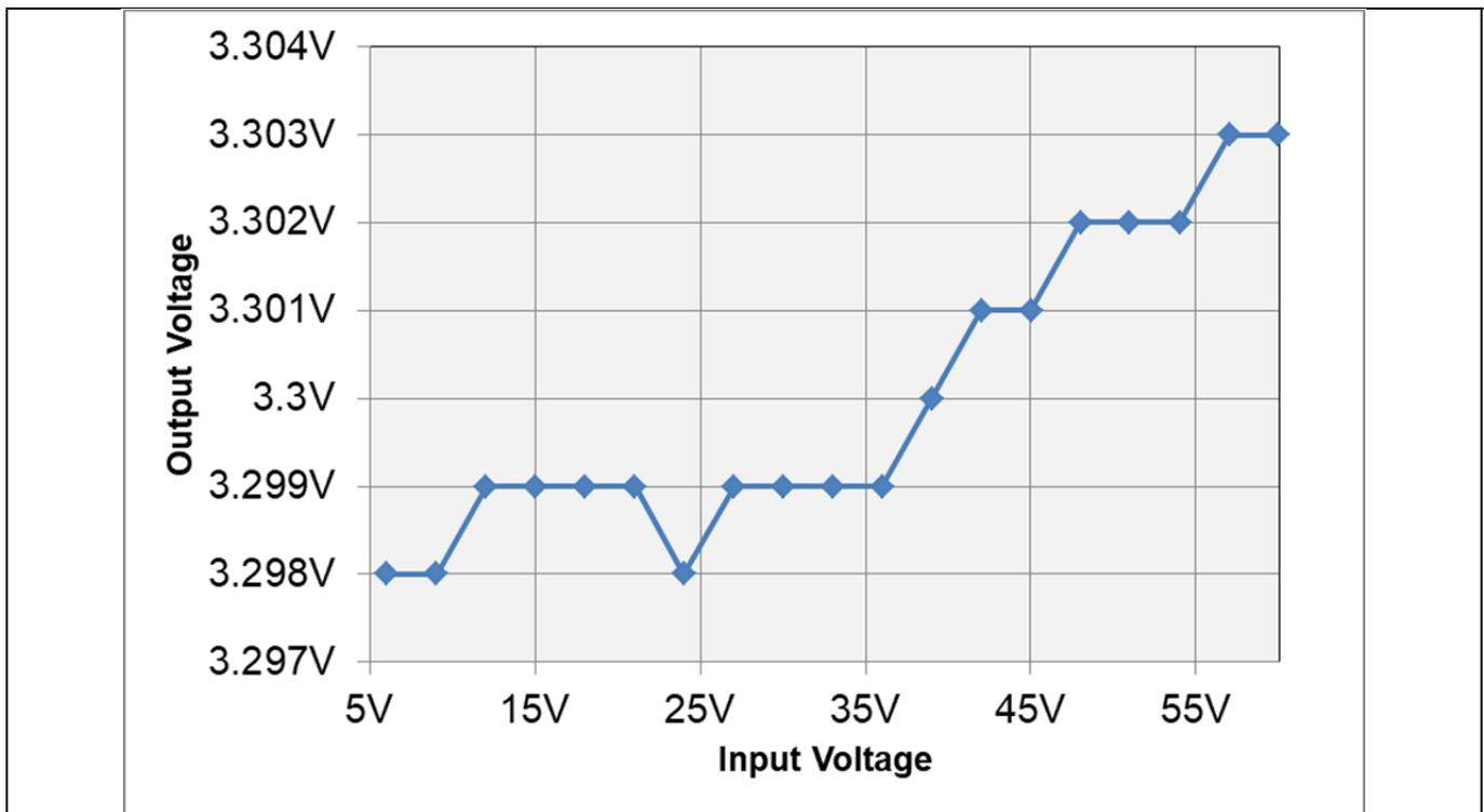
Figure 10. Output Voltage vs Input Voltage for the 3.3 V Output
