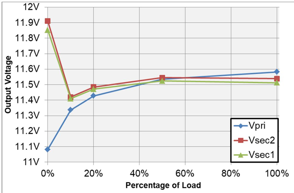
Figure 5. Output Voltage vs Load for the 11 V Outputs
