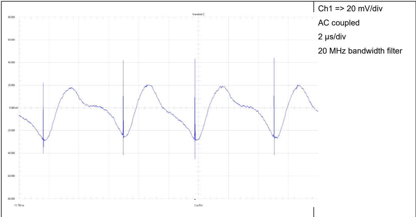
**Figure 26. Input Voltage Ripple 6 V**
