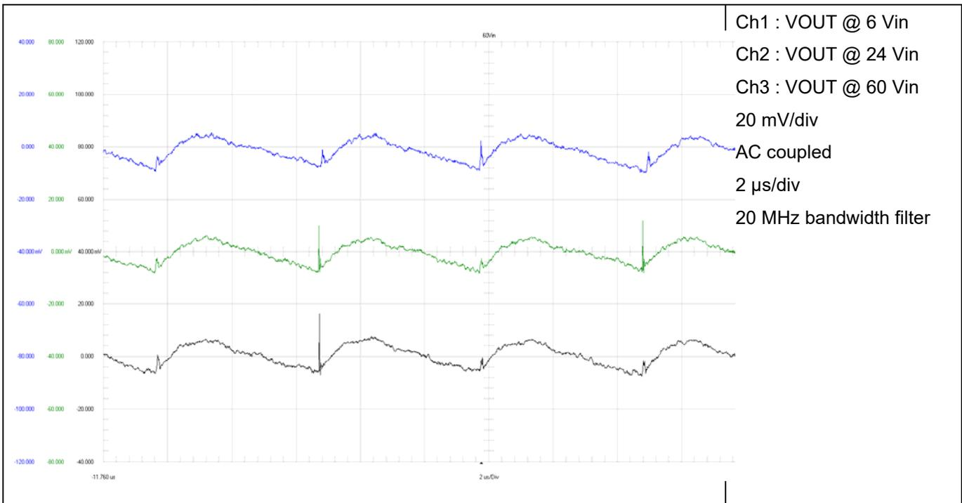
**Figure 24. 11 V Output Voltage (Isolated Vo1)**
