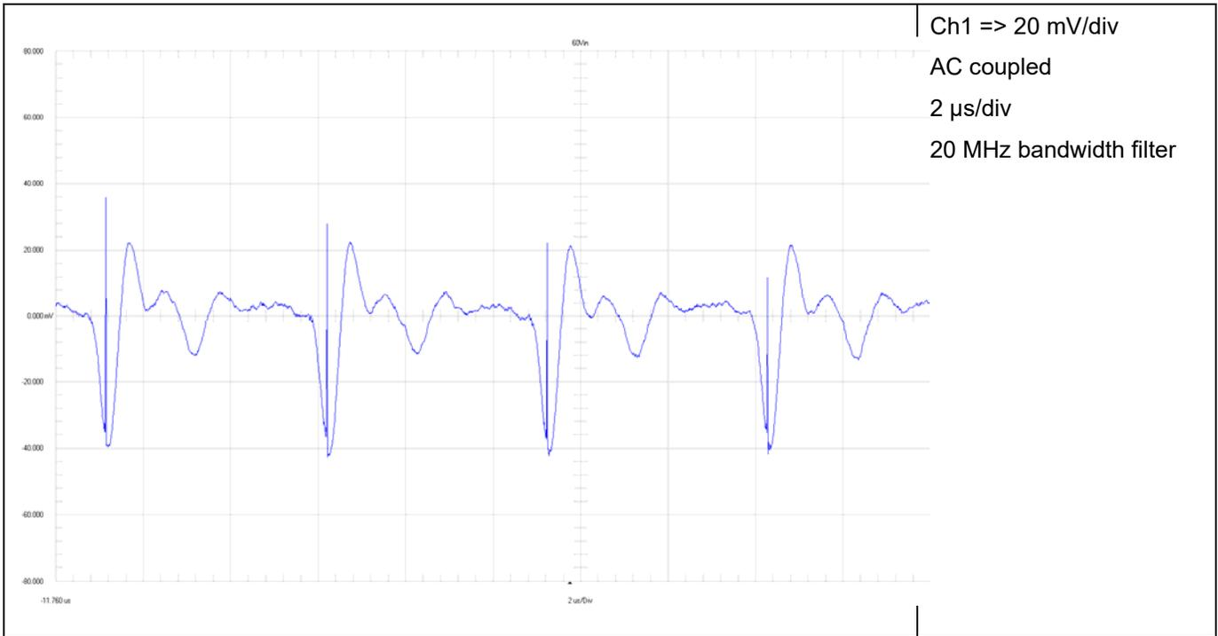
**Figure 28. Input Voltage Ripple 60 V**
