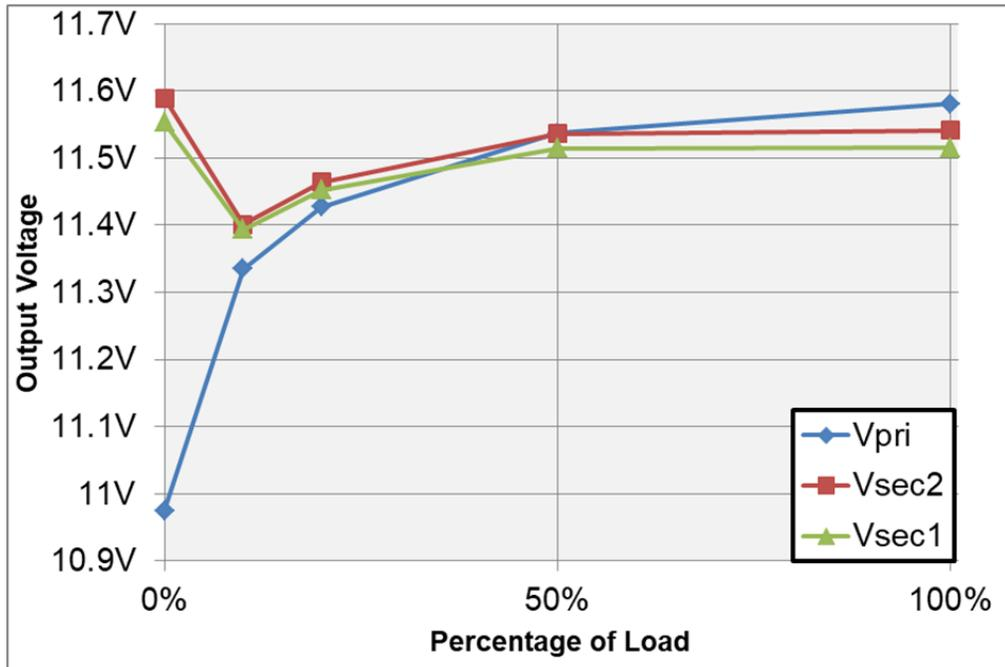
Figure 3. Output Voltage vs Load for the 11 V Outputs
