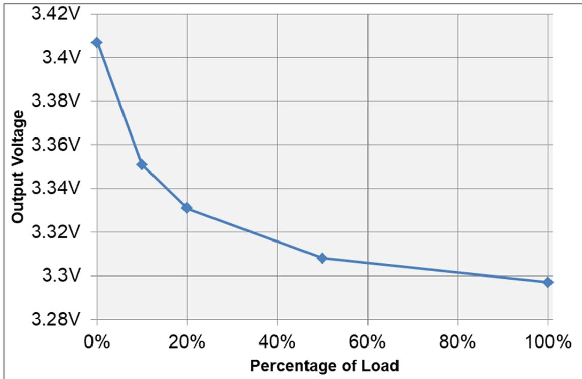
Figure 6. Output Voltage vs Load for the 3.3 V Output
