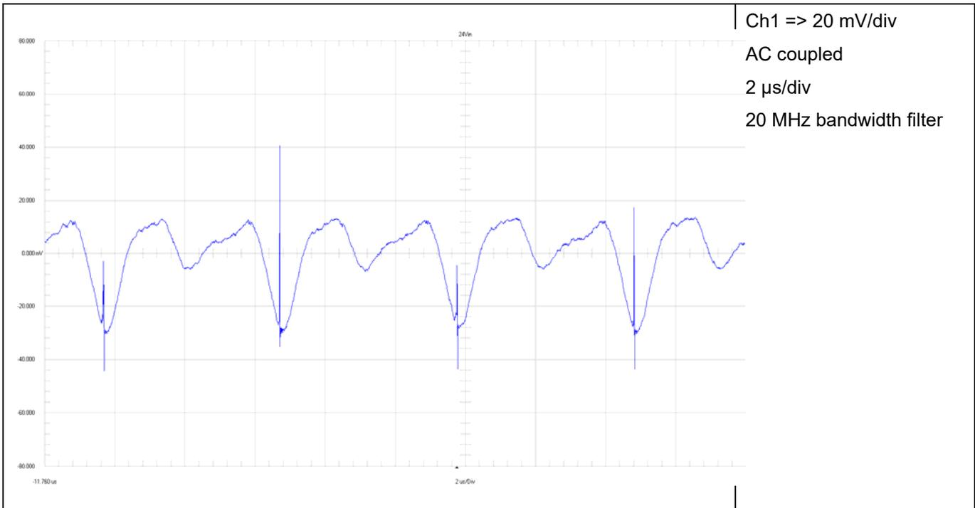
**Figure 27. Input Voltage Ripple 24 V**
