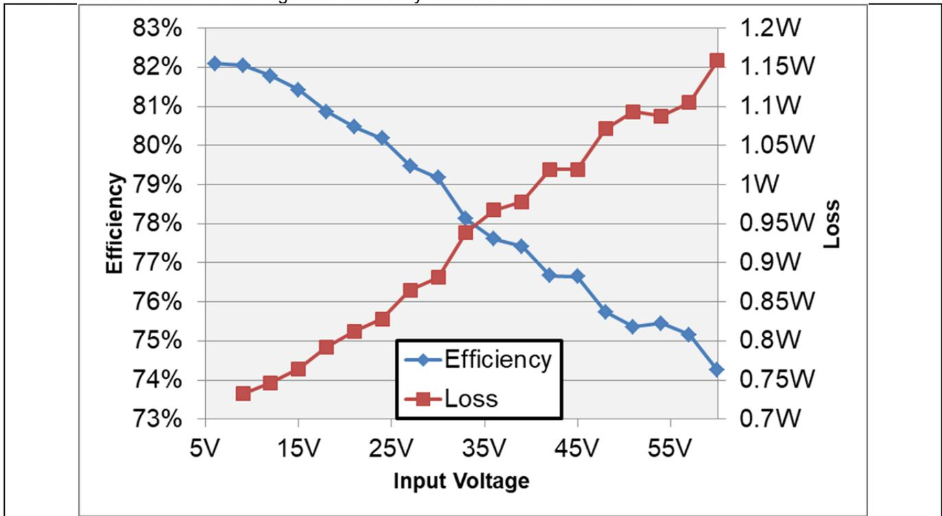
Figure 11 Input Voltage vs Efficiency and Loss
