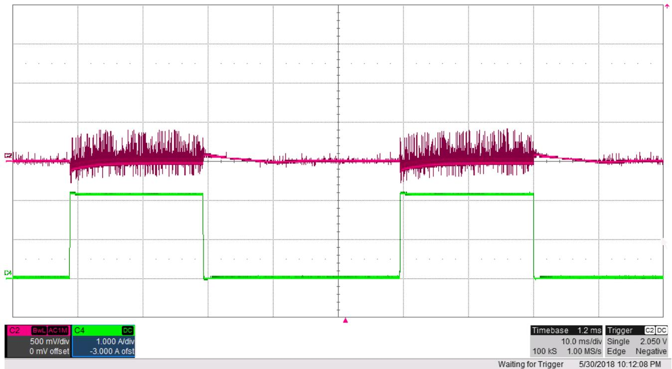
**Figure 15. 120 VAC Load Transient**
