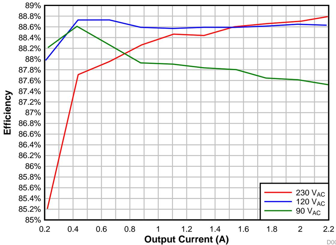
Figure 1. Efficiency Graph
