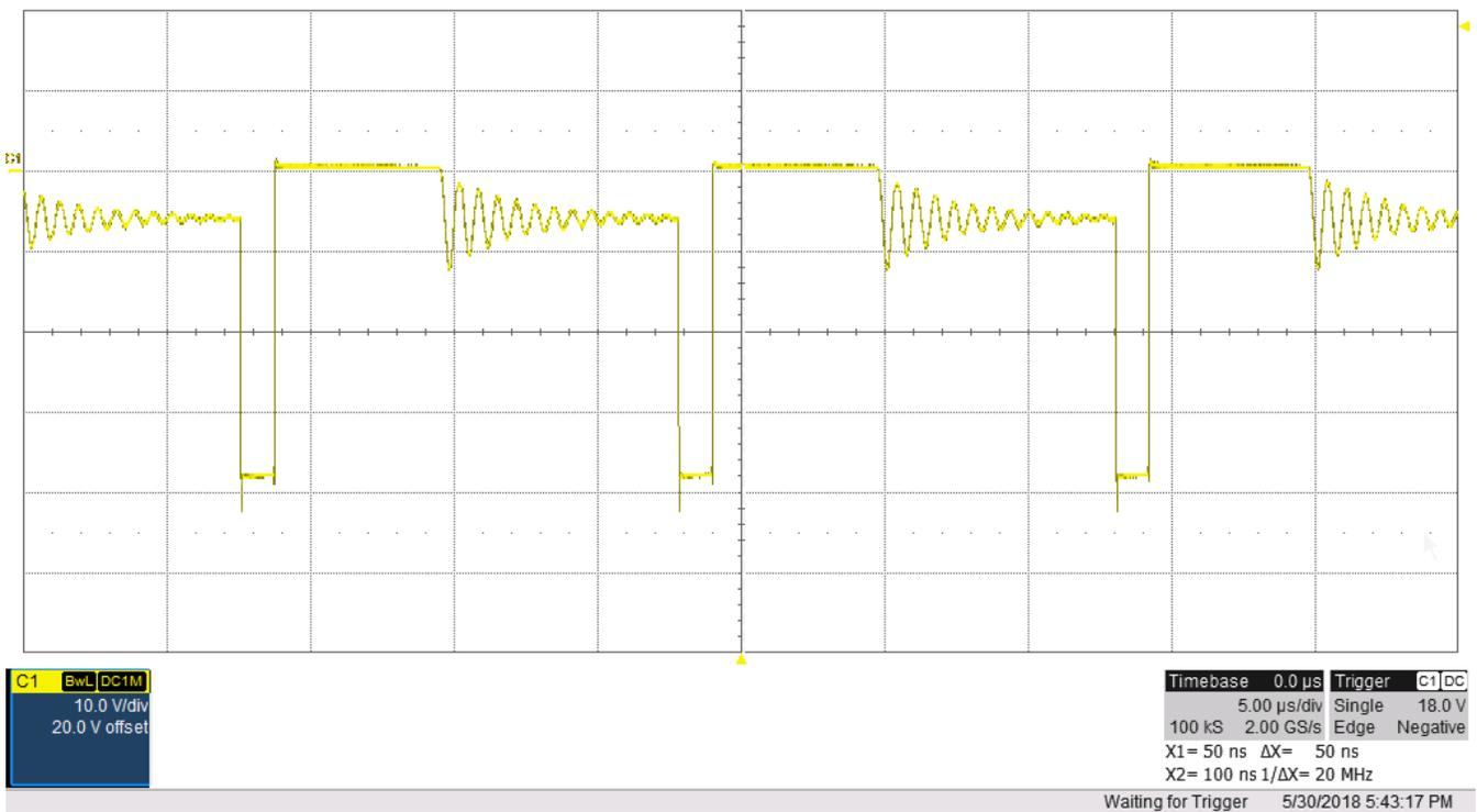
Figure 10. Voltage Across 6 V Line Rectifier (D1)
