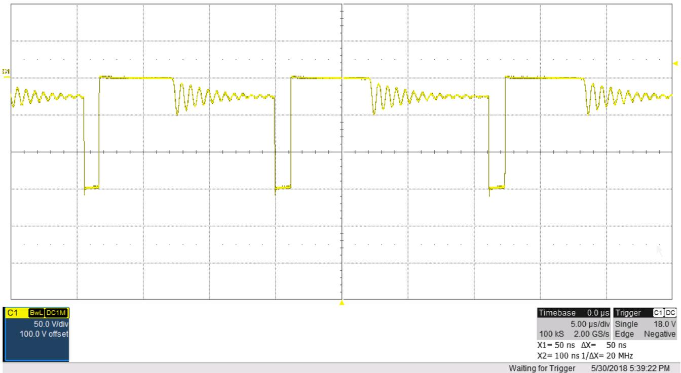
Figure 9. Voltage Across 24 V Line Rectifier (D2)
