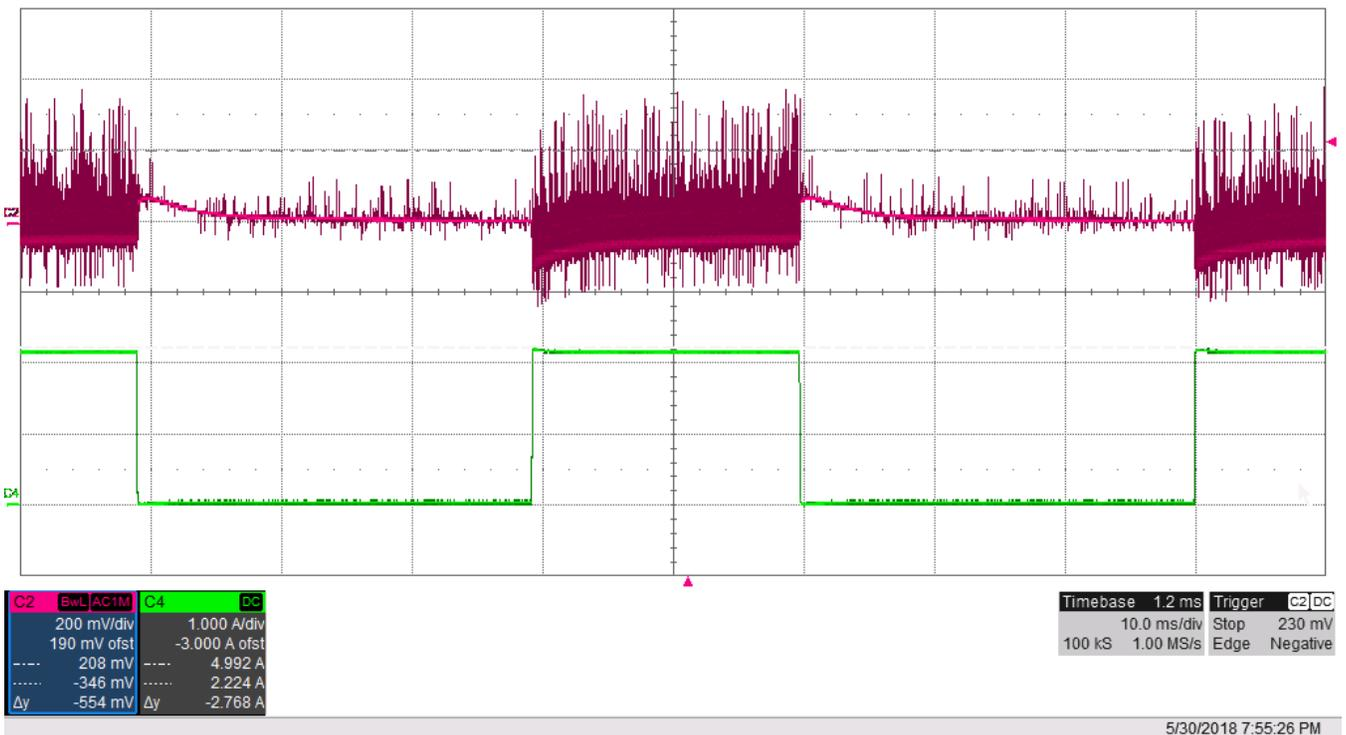
Figure 14. 230 VAC Load Transient
