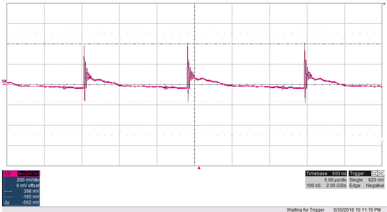
Figure 12. 120 VAC Voltage Ripple on 24 V Line
