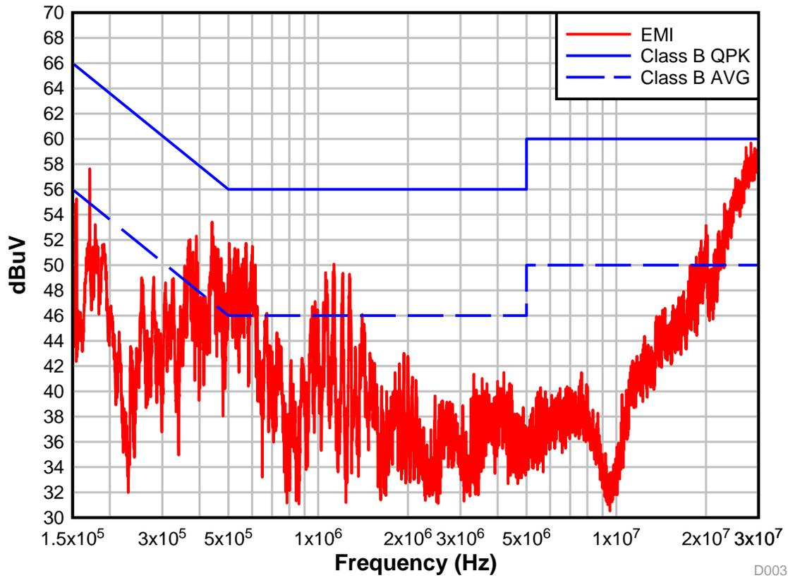
Figure 21. Peak Detector, Max-Hold - 120 VAC/50 Hz Input, Full Load
