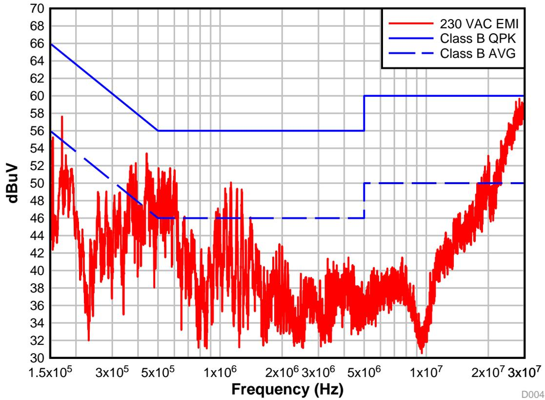
Figure 20. Peak Detector, Max-Hold - 230 VAC/50 Hz Input, Full Load
