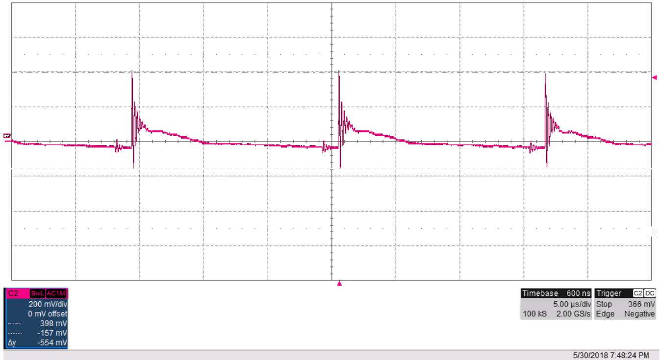
Figure 11. 230 VAC Voltage Ripple on 24 V Line
