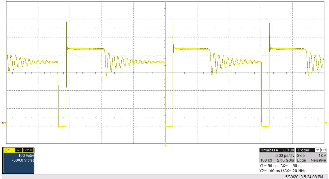
**Figure 8.  $V_{DS}$  of Primary Side MOSFET (Q1)**
