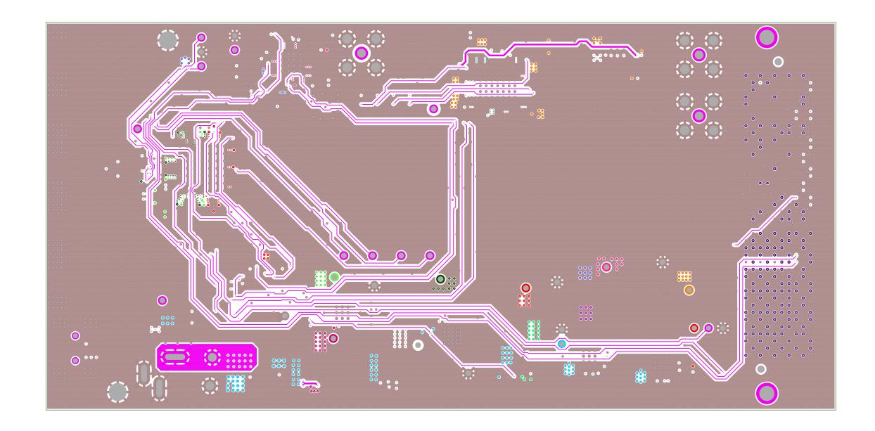
TEXAS INSTRUMENTS, INC. ADC3XRFXXEVM PCB REV E LAYER 4 - GND
