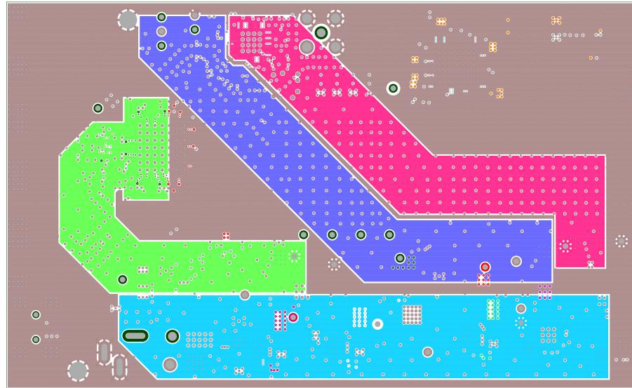
TEXAS INSTRUMENTS, INC. ADC3XRFXXEVM PCB REV E LAYER 3 - POWER
