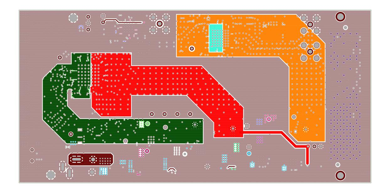
TEXAS INSTRUMENTS, INC. ADC3XRFXXEVM PCB REV E LAYER 6 - POWER/SIGNAL
