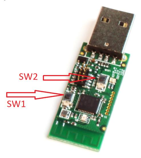
Pressing **SW2** on the dongle disconnects any active connection between the dongle and an advanced remote.
