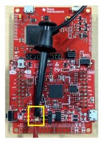
Figure 13. Current Measurement Tool Connection to CC3120 Device
