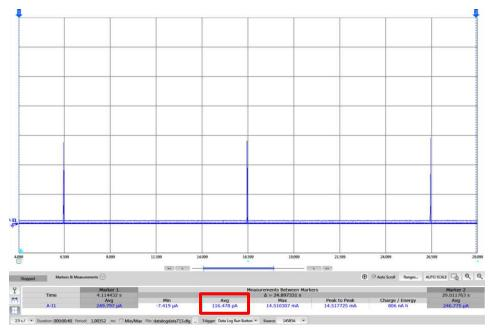
Figure 31. CC3120 Device in LPDS Mode
