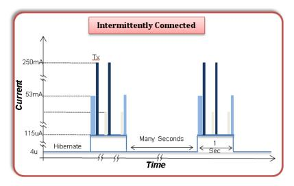
Figure 3. Intermittently Connected Test Case
