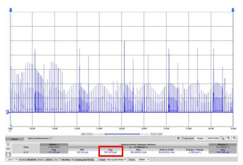
Figure 40. CC3220SF Device in Always Connected Mode (UDP)
