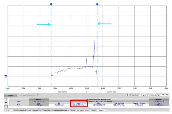
Figure 12. Average Current Measurement With DC Power Analyzer
