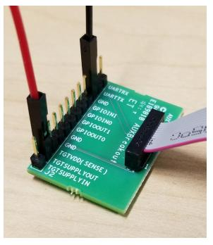
Figure 22. Breakout Board Connection
