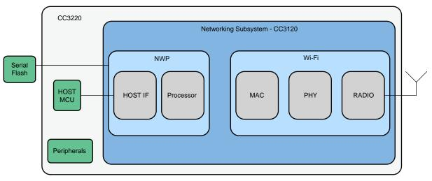
Figure 1. CC3120 and CC3220 Device Block Diagram
