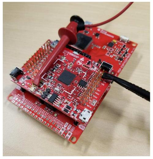
Figure 9. DC Power Analyzer Connection to CC3120 Device
