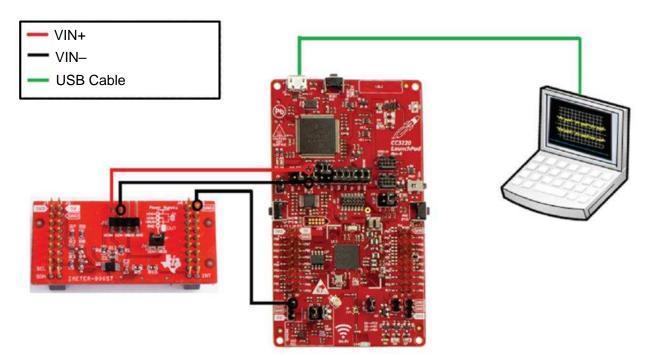
Figure 15. IMETER-BOOST Test Setup
