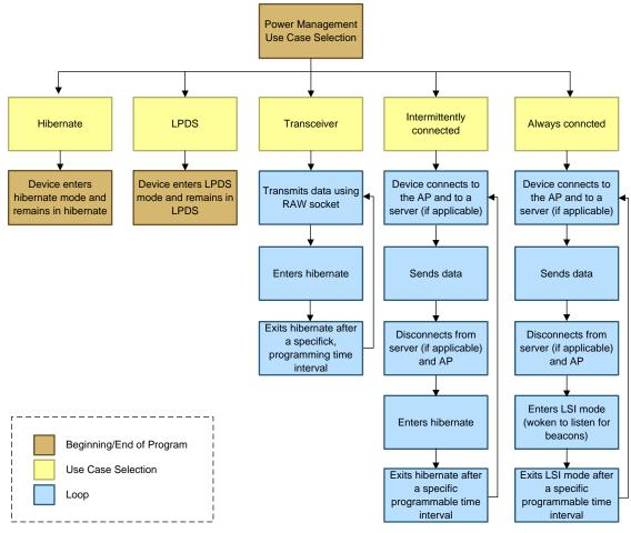
Figure 8. Power Management Use-Case Selection Flowchart
