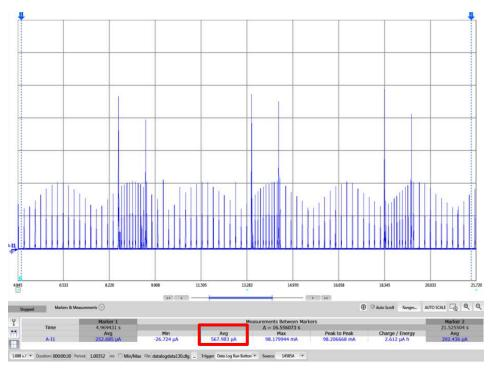
Figure 39. CC3120 Device in Always Connected Mode (UDP)
