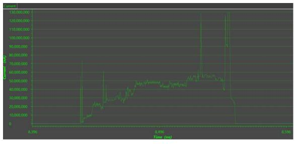
Figure 28. Average Current Measurement With EnergyTrace™
