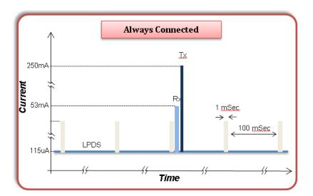
Figure 4. Always Connected Test Case
