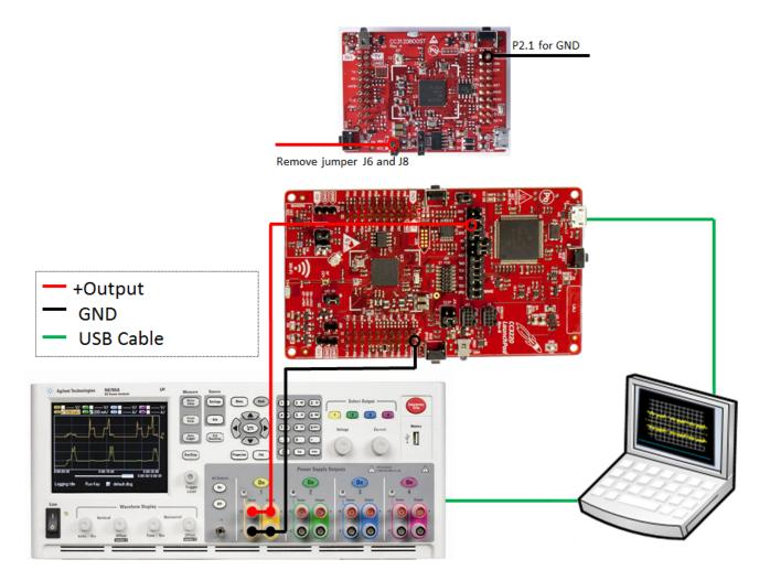
Figure 11. DC Power Analyzer Test Setup
