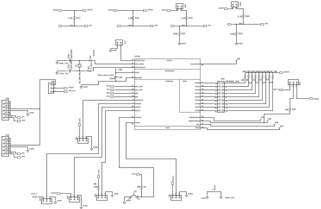
**Figure 2. Control and Communication Schematic**
